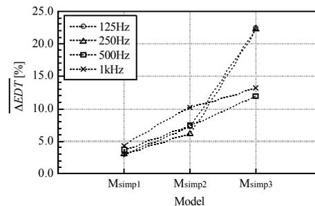
Figure 5: Mean of relative errors  $\overline{\Delta EDT}$  between original model and simplified models.
