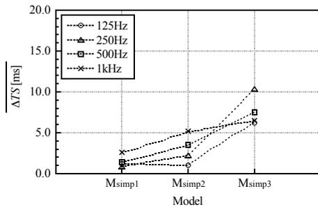
Figure 8: Mean of absolute errors  $\overline{\Delta TS}$  between original model and simplified models.
