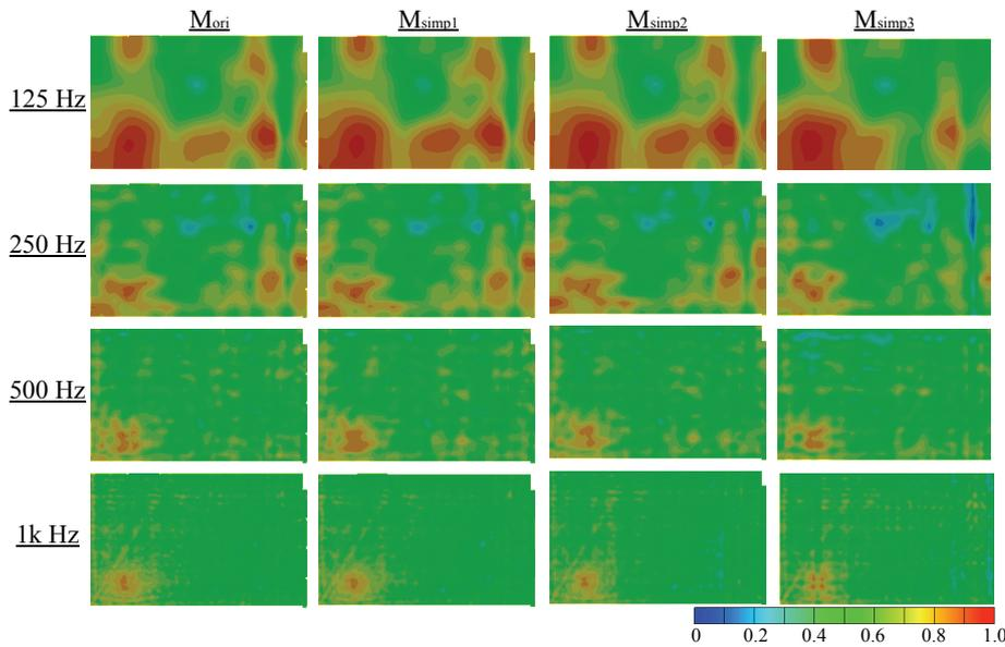
Figure 7: Comparison of spatial distributions of  $D_{50}$  calculated using four models.
