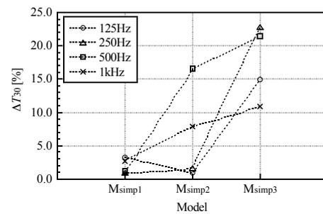
Figure 4: Relative errors of  $T_{30}$  between original model and simplified models.
