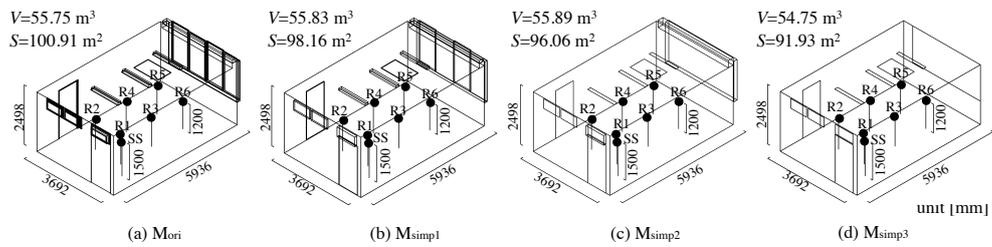
Figure 1: Schematic drawings of four office models to be analyzed. The dots, R1~R6 represent computed points of sound pressure responses.
