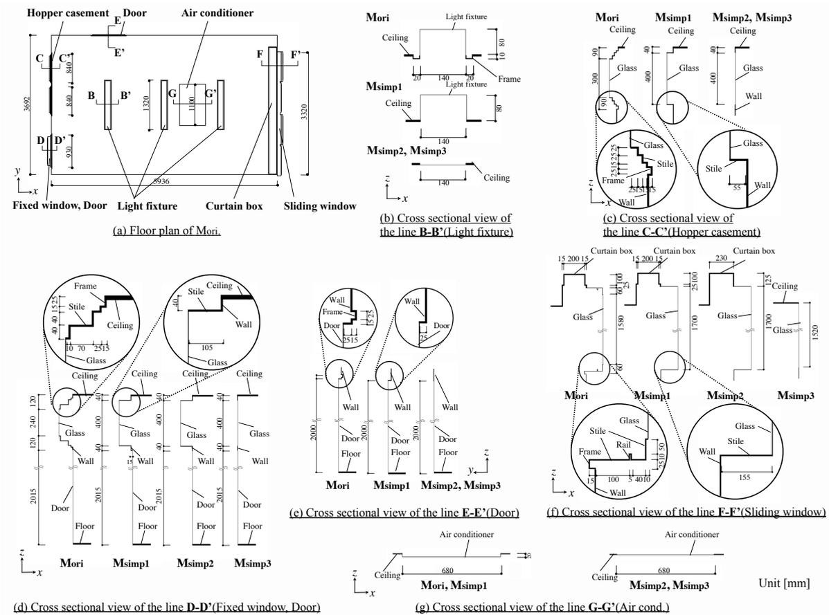
Figure 2: Floor plan of  $M_{ori}$  and cross sectional views of building elements of four office models.
