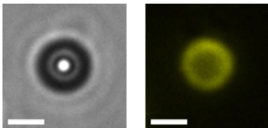
**Figure 2.** Bright field and corresponding fluorescence image of a phospholipid microbubble. Scale bar indicates 2  $\mu\text{m}$ .
