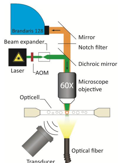
**Figure 1.** Schematic view of the experimental setup.
