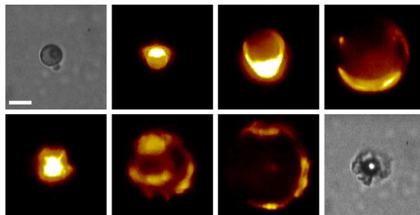
**Figure 5.** Frames from a fluorescence recording of vapor bubble oscillations due to high intensity laser illumination. The bright field images show the microcapsule before and after the laser-excited oscillations. Scale bar indicates 5  $\mu\text{m}$ .
