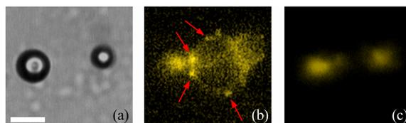
**Figure 4.** (a) Bright field image from the first recording before ultrasound. (b) Fluorescence image from the second recording at -500kPa, red arrows indicating high dye concentration at bubble wall. (c) Fluorescence image of dye residue at initial bubble positions from the sixth recording. Scale bar indicates 5  $\mu\text{m}$ .
