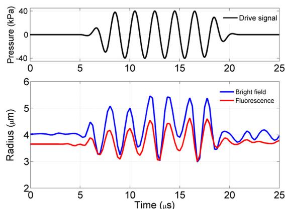
**Figure 3.** Radius time curve of an oscillating microbubble, recorded first in bright field (blue curve) and with a delay of 100ms in fluorescence (red curve).
