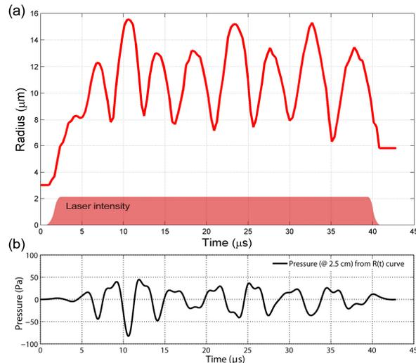
**Figure 6.** (a) Radius time curve of a microcapsule illuminated with a laser intensity of  $1 \text{ MW/cm}^2$ . (b) Predicted pressure field of the vapor bubble at 2.5 cm.
