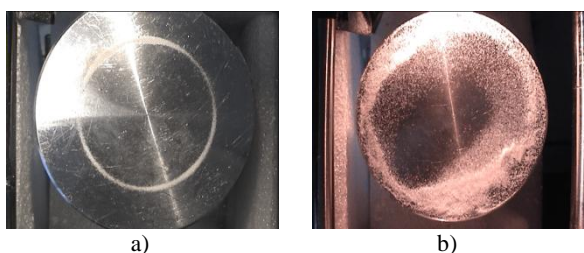
Figure 9. Natural resonance frequencies attained on the circular plate 70 mm diameter, 52.27 mm thickness; a) particles clumping at f=40.03 kHz; b) particles clumping at f=40.07 kHz.
