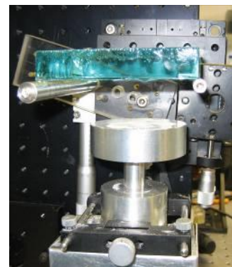
Figure 8. a) Assembly of the test plate, drive and reflector; b) attachment of test disc to the stepped horn; c) photograph of assembly and micromanipulators.
