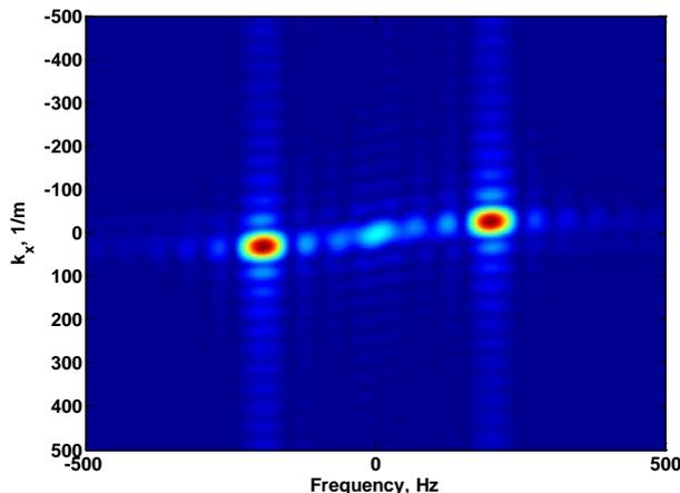
Fig. 4. Two-dimensional Discrete Fourier Transform of the data presented in Figure 3 yields the k-space map that can be used for calculation of the Lamb wave speed at the given excitation frequency.
