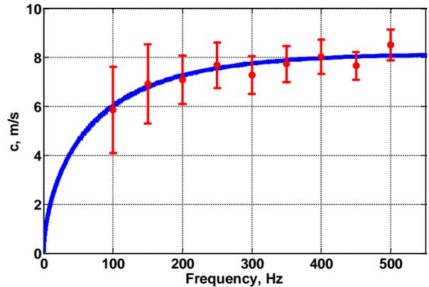
Fig. 5. Lamb wave ABAQUS simulations: Lamb wave dispersion equation in blue is fitted to the finite element method Lamb wave speeds  $\pm$  one standard deviation shown in red.
