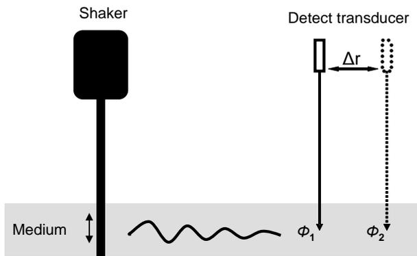
Fig. 1. Principle of Lamb Wave SDUV: a mechanical actuator (shaker) is the source of force that induces harmonic shear wave propagation in medium of interest; the motion is measured by a pulse echo (detect) transducer.
