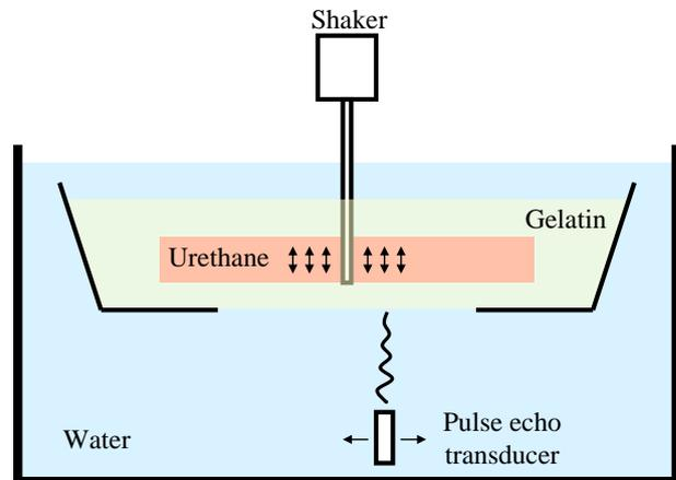
Fig. 2. Experimental set up for the Lamb Wave SDUV approach: a mechanical actuator (shaker) was used to excite shear waves in the urethane rubber sample; pulse echo transducer was used to detect the motion. The gelatin was used as a stabilizer.
