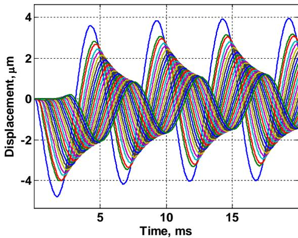
Fig. 3. ABAQUS displacement at 28 different points along the line of cylindrical wave propagation in an isotropic plate submerged in water, 1 mm apart, at the excitation frequency of 200 Hz.
