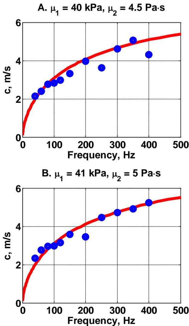
Fig. 6A and 6B. Urethane rubber: experimentally obtained shear wave dispersion curves are shown as blue circles. Lamb wave model (red line) was fitted to the data to obtain the values of elasticity and viscosity  $\mu_1$  and  $\mu_2$ .
