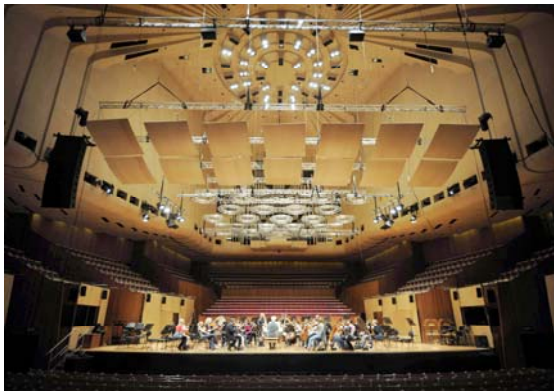
Figure 15. Prototype array, showing reconfigured clouds supplemented with additional plywood panels
