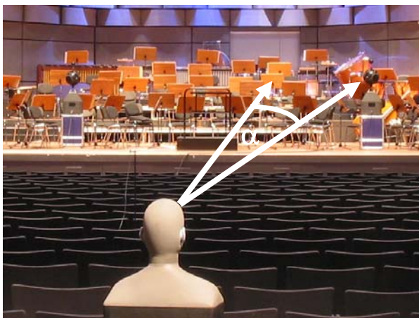
Figure 2 Artificial head (ITA [5]) and dodecahedron loudspeakers (ITA [6]) during measurement with a misalignment of \alpha
