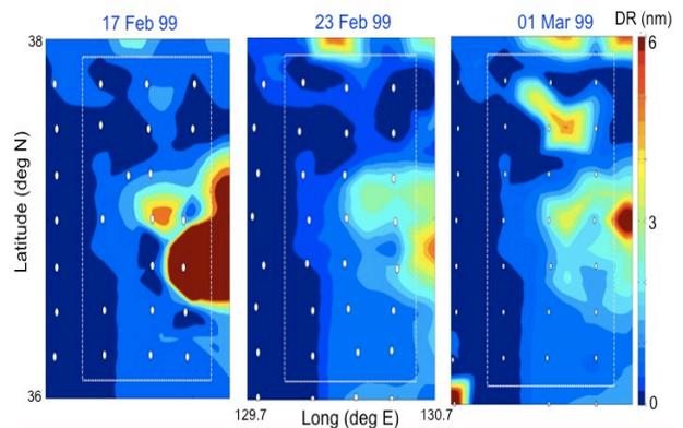
**Figure 3.** Ground-truth active sonar detection ranges on 17 Feb (left), 23 Feb (center), and 1 Mar (right) for source and receiver at 300-m depth and target at 20-m depth.
