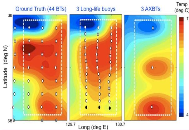
**Figure 2.** Temperature assimilation results at 100-m depth on 1 Mar for ground-truth (left), 3 SWEM buoys (center), and 3 AXBTs (right).
