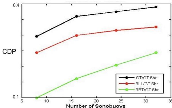
Figure 6. CDP results for 8, 16, 24, and 32 sonobuoys using ground-truth, 3 SWEM long-life, and 3AXBT environments.
