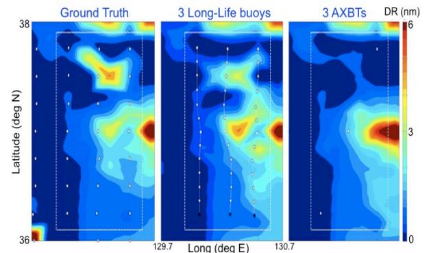
**Figure 4.** Detection ranges for a monostatic active system at 750 Hz with source and receiver at 300-m depth and target at 20-m depth.
