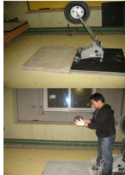
Figure 3. Floor impact sound measurement in reverberation chamber with bang machine and impact ball
