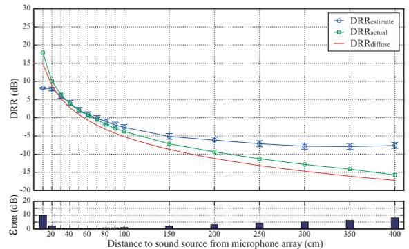
Figure 4: Comparison between estimated and actual DRR in simulated room. In upper graph, lines with circles and squares show  $\text{DRR}_{\text{estimate}}$  and  $\text{DRR}_{\text{actual}}$ , respectively. Other line shows principle-based DRR in diffuse sound field, which helps to determine distance of actual reverberation from completely diffuse field. Log DRR difference between  $\text{DRR}_{\text{estimate}}$  and  $\text{DRR}_{\text{actual}}$  is shown in lower graph.
