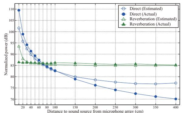
Figure 5: Comparison between estimated and actual power spectra of direct sound and reverberation, which are denoted by circular and triangular markers, respectively.
