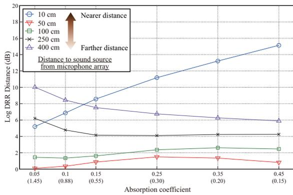
Figure 9: Log DRR difference measured at edge of room. Each line shows log DRR difference measured at particular distance to sound source from microphone array. Parenthetic values in x-axis show approximate reverberation time corresponding to each absorption coefficient.
