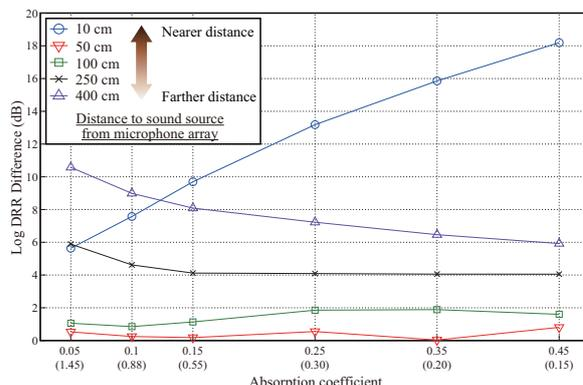
Figure 7: Log DRR difference measured for different reverberation times. Each line shows log DRR difference measured at particular distance to sound source from microphone array. Parenthetic values in x-axis show approximate reverberation time corresponding to each absorption coefficient.
