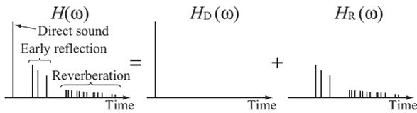
Figure 1: Decomposition of transfer function.
