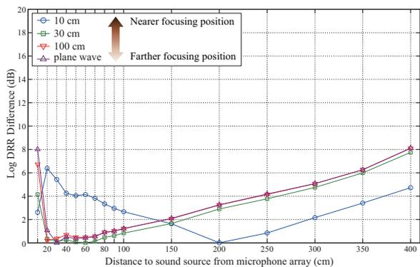
Figure 6: Log DRR difference calculated when spatial correlation of direct sound is modelled by assuming spherical wave. Each line shows log DRR difference measured for changed focusing positions. For comparison, line with upward triangles shows log DRR difference of estimated DRR using plane wave assumption.
