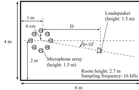
Figure 3: Positions of microphone array and speaker in simulated reverberant room.
