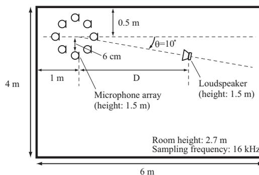
Figure 8: Position of microphone and sound source applied to evaluate influence of early reflection. Both microphone array and speaker are parallel shifted from basic position shown in Fig. 3.
