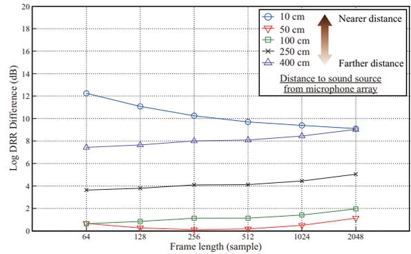
Figure 14: Effect of frame length on calculation for estimated DRR. Each line shows log DRR difference measured at particular distance to sound source from microphone array.
