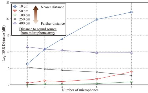
Figure 13: Errors in estimated DRR for different numbers of microphones. Each line shows log DRR difference measured at particular distance to sound source from microphone array.
