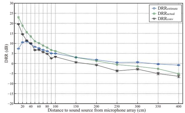
Figure 12: Evaluation of DRR estimation compared to conventional method (little reverberation condition).
