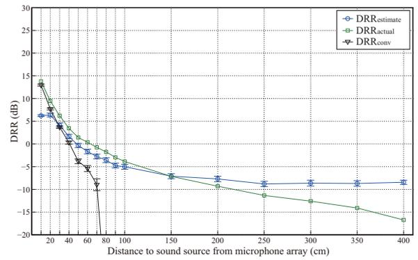
Figure 11: Evaluation of DRR estimation compared to conventional method (highly reverberant condition).
