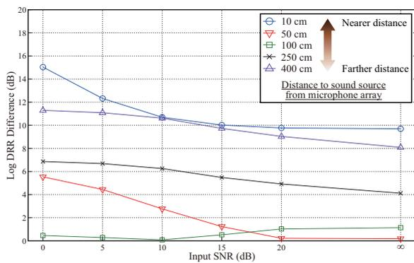
Figure 10: Influence of spatially uncorrelated noise for estimated DRR. Each line shows log DRR difference measured at particular distance to sound source from microphone array.
