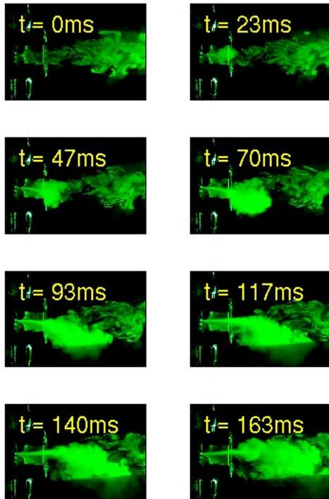
**Figure 6.** Visualization of the unsteady flow through a rigid rounded glottal replica in forced motion. An asymmetry is generated by moving only one replica while the other one stays steady.
