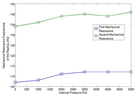
**Figure 4.** Extracted first and second resonance from mechanical frequency response. The internal pressure,  $P_{cin}$  is varied.
