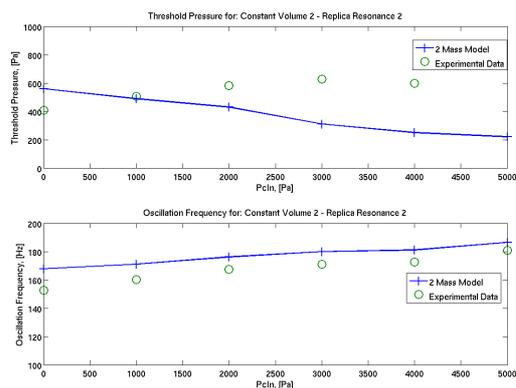
**Figure 8.** Measured (o) and simulated (+) onset threshold pressure [Pa] and associated oscillation frequency [Hz] in case the volume (in the intermediate layer) is held constant.
