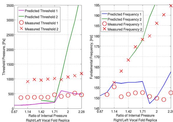
**Figure 7.** Measured (symbols) and predicted (lines) threshold pressure and frequency of oscillation as a function of the ratio of the water pressure inside each vocal fold replica (1 being the mechanically symmetric case)
