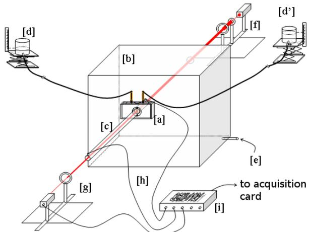
Figure 2. Experimental set-up: a: vocal folds replica, b: reservoir, c: acoustical resonator, d and d': water column, e: air supply, f: laser beam, g: photodiode, h: pressure sensors, i: daq.
