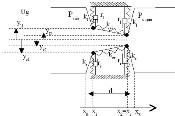
Figure 1. Two-mass model for the vocal folds
