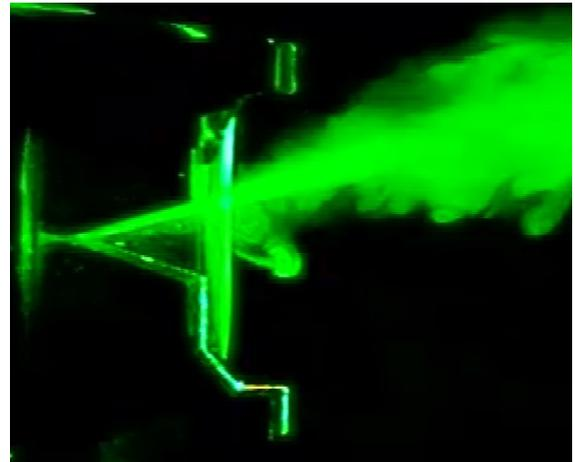
**Figure 5.** Visualization of the Coanda effect in the case of a steady flow through a rigid glottal replica having a 30° angle of divergence. Minimum glottal aperture is  $h=0.6\text{mm}$  and flow rate is 15l/min.
