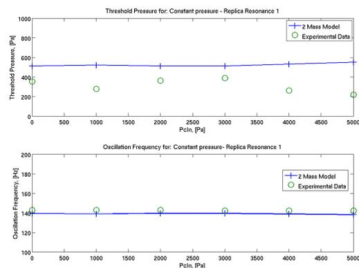
**Figure 8.** Measured (o) and simulated (+) onset threshold pressure [Pa] and associated oscillation frequency [Hz] in case the internal pressure (in the intermediate layer) is held constant.
