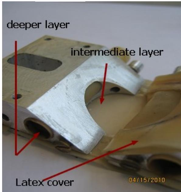
**Figure 3.** Internal structure of the inhomogeneous vocal fold replica. The deeper layer consists of a latex tube filled with water at pressure  $P_{cin}$ , the intermediate layer, filled with water at a different pressure, is covered by a thin latex cover. (removed for the picture)
