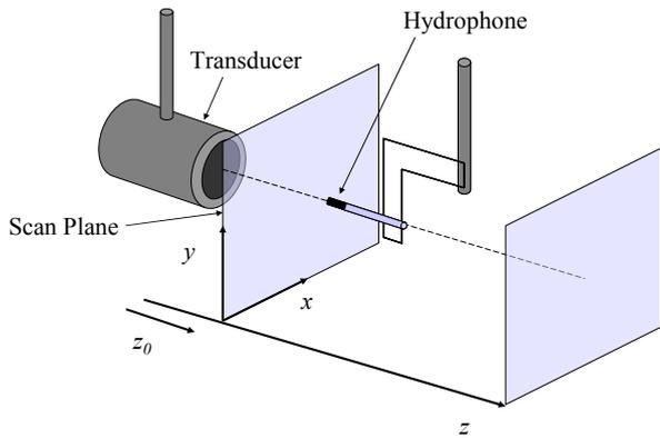
**Figure 1.** Experimental arrangement for making 2-D hydrophone scans in the near-field of a transducer.
