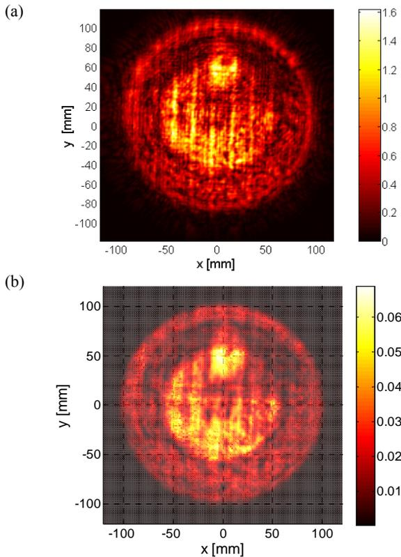
**Figure 3.** Results for (a) pressure amplitude measured at 10 mm from the transducer face and (b) direct measurement of the surface velocity amplitude using a scanning LDV (linear scale).
