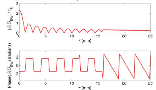
**Figure 7.** Velocity artefact (apparent velocity – true velocity) for the results presented in Figure 6. All amplitudes and phases are expressed relative to those of the true surface velocity over the radiating area.
