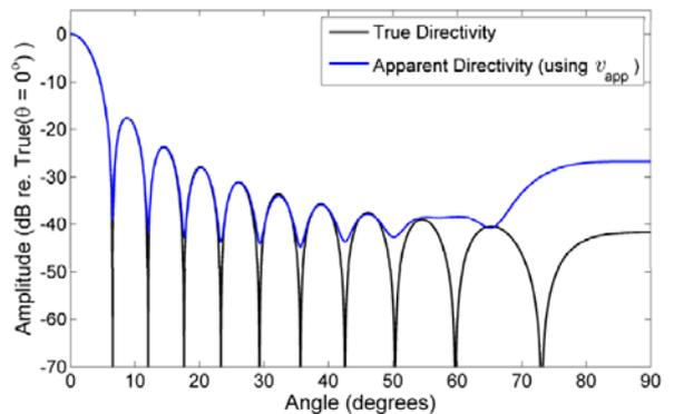
**Figure 8.** Predicted far-field directivities calculated from the simulated apparent velocity distribution for a 15.9 mm radius, 500 kHz circular piston transducer. The true directivity is shown for comparison.
