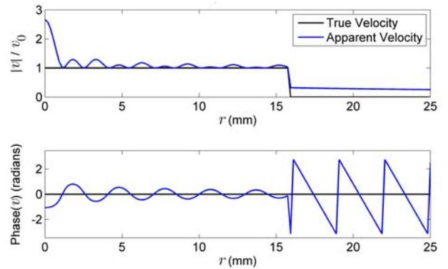
**Figure 6.** Simulated steady-state apparent velocity and true surface velocity for a 15.9 mm radius circular piston source. All amplitudes and phases are expressed relative to those of the true surface velocity over the radiating area.
