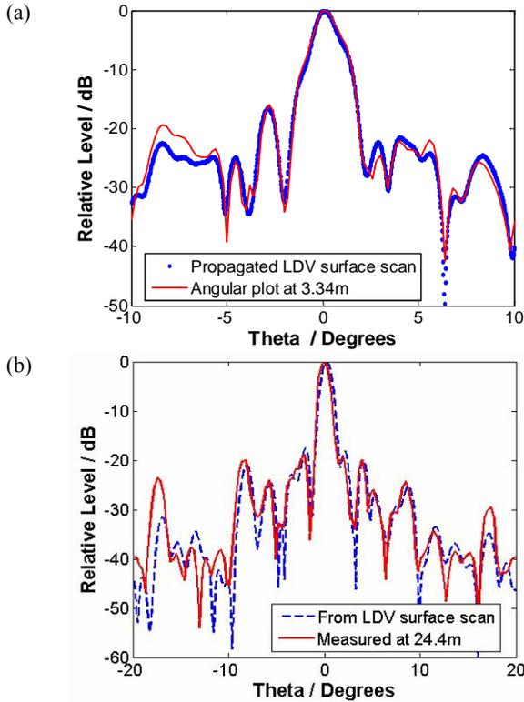
**Figure 5.** Measured beam plots for 500 kHz transducer at (a) 3.34 m and (b) 24.4 m. Measurements are compared with the results predicted by linear propagation of the LDV scan data.
