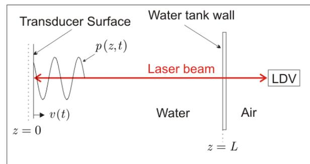
**Figure 2.** Basic LDV geometry, showing an acoustic pulse having travelled part way to the tank boundary.
