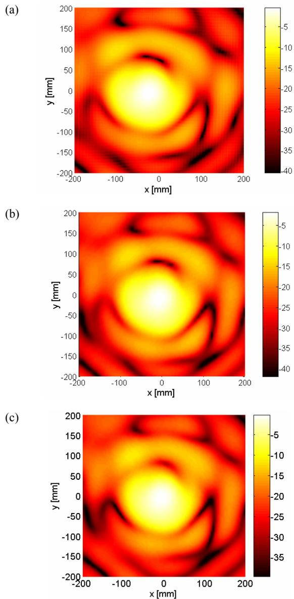
**Figure 4.** Normalised pressure amplitude results (in dB) in the  $xy$ -plane for the 500 kHz transducer at 3.34 m showing: (a) forward-propagated pressure field from 10 mm, (b) direct measurement at 3.34 m, and (c) forward-propagated optical LDV surface velocity measurements.
