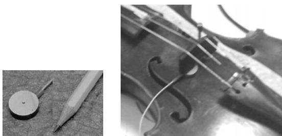
**Figure 2.** Micro load cell under the bridge
