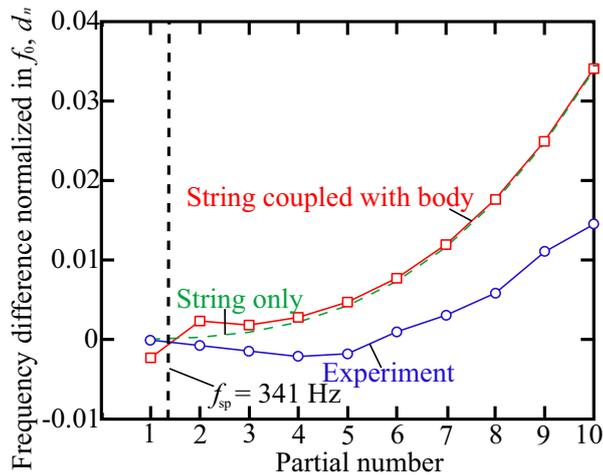
Figure 7. Inharmonicity of vibration modes (B3 246.9 Hz 2nd)
