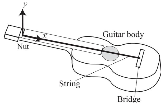
**Figure 1.** Definition of coordinate system
