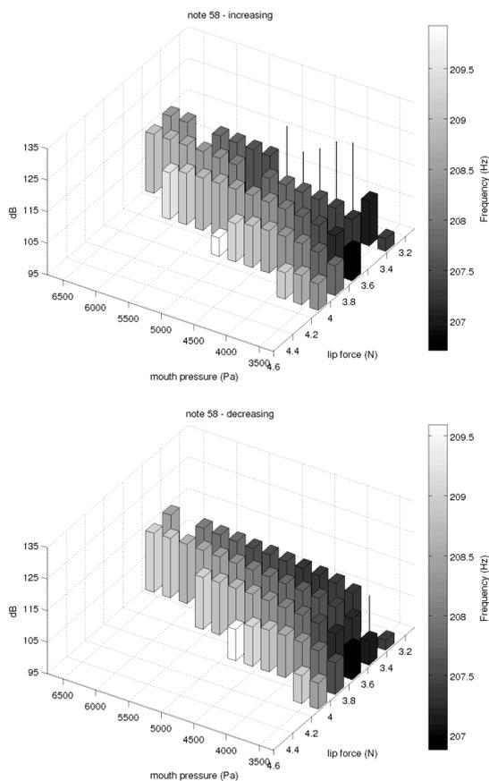
**Figure 4:** Plots of playing frequency as a function of air pressure and lip force  $f(P,F)$  for the note (written A#3). In this run,  $F$  was held constant while  $P$  was increased (top) or decreased (bottom). Narrow columns are ‘wrong’ notes produced with this fingering, usually squeaks.
