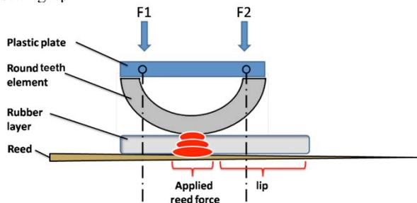
**Figure 3.** Forces  $F_1$  and  $F_2$  are applied to the elements that take the roles of teeth and lips to press against the reed.
