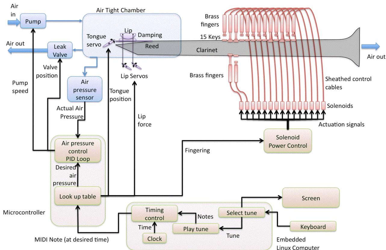
Figure 2. A schematic of the clarinettist showing the mechanisms and controllers. Not to scale.
