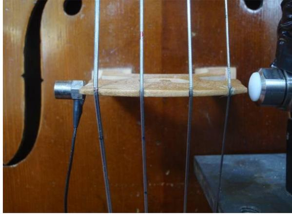
**Figure 6.** Experimental modal identification of the cello body through impact tests.
