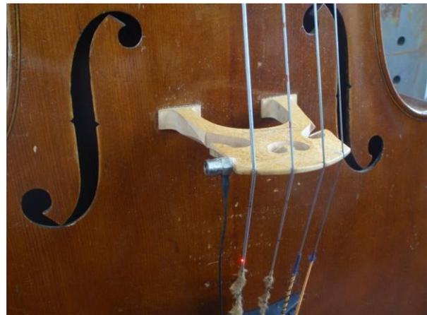
**Figure 4.** Set-up for the measurement of the bridge transverse dynamical responses and of the “dead” string-side motion.
