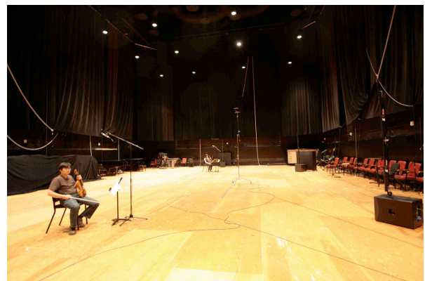
Figure 19. The arrangement of two musicians in the scoring stage of MMR studio with the virtual acoustics support added via four line-array loudspeakers. Musicians are seated at position 3 (13 m apart) in the 'Hall' configuration.
