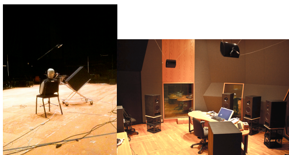
Figure 10. Source/receiver set up for measuring binaural impulse responses in position 1 (left); and listening environment for evaluating recorded performances (right)
