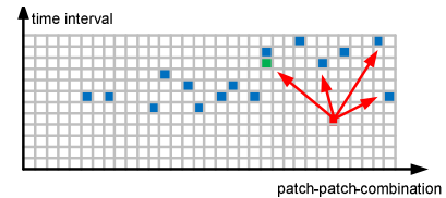
c) re-unification of two sound particles by adding a sound particle to an already set matrix element (green)
