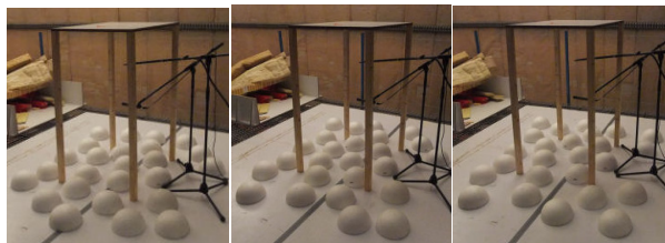
Figure 17. View of different 25 cm diameter semi-sphere diffuser arrangements (Diff 1, Diff 2, Diff 3) for a coverage rate of 31 %.
