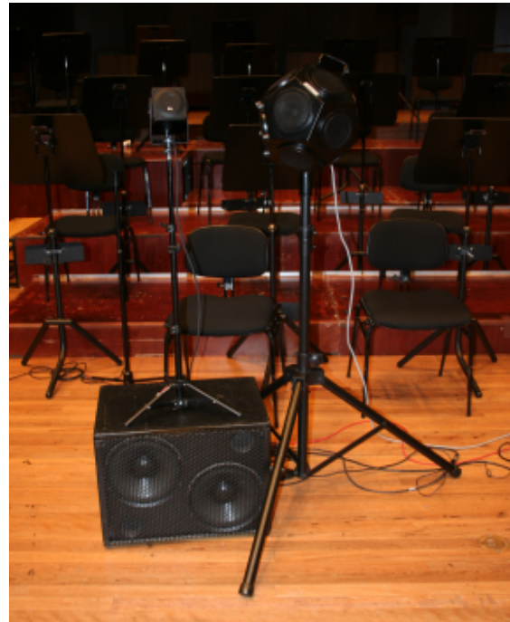
Figure 3. Photograph of Meyer Sound MM-4XP with UMS-1P subwoofer next to a B&K 4292 Omnidirectional sound source.
