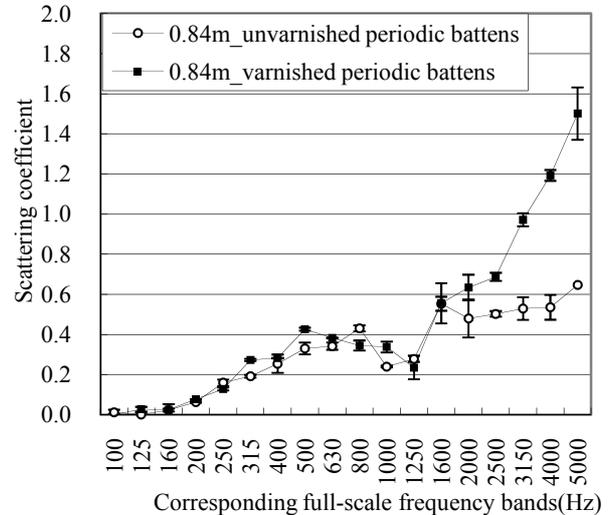
**Figure 10.** Scattering coefficients of the unvarnished and varnished periodic battens (sample without an edge strip, sample diameter 0.84 m, air gap 105 mm).
