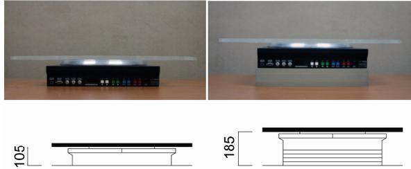
**Figure 4.** The variations of the air gap below the turntable ranged from 105 mm to 185 mm.
