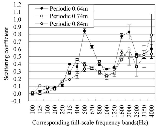
**Figure 6.** Scattering coefficients of unvarnished periodic battens, measured with three different sample diameters (Sample without edge strip, air gap 105 mm).
