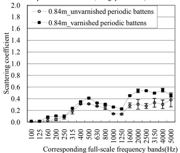
**Figure 11.** Scattering coefficients of the unvarnished and varnished periodic battens (sample with an edge strip, sample diameter 0.84 m, air gap 105 mm).
