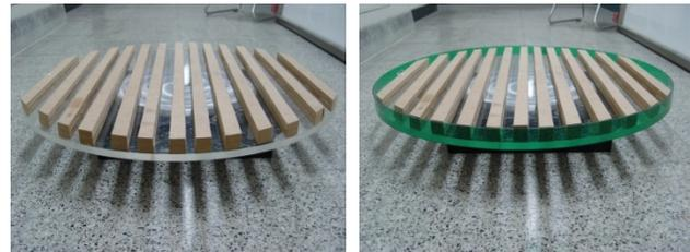
**Figure 2.** Samples of the periodic baffens (left: samples without an edge strip, right: samples with an edge strip).
