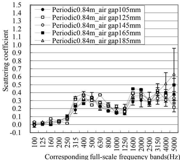
**Figure 9.** Scattering coefficients of unvarnished periodic battens, measured with five different air gaps (sample with an edge strip, sample diameter 0.84 m).
