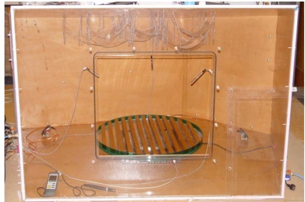
**Figure 1.** A 1/5 scale model of the reverberation chamber.
