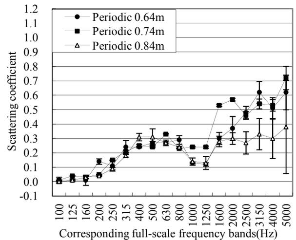
**Figure 7.** Scattering coefficients of unvarnished periodic battens, measured with three different sample diameters (Sample with an edge strip, air gap 105 mm).
