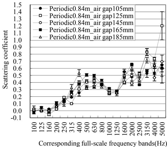
**Figure 8.** Scattering coefficients of unvarnished periodic battens, measured with five different air gaps (sample without an edge strip, sample diameter 0.84 m).
