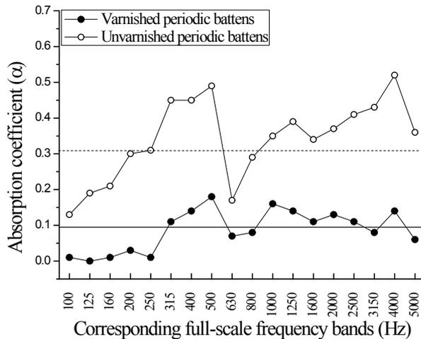
**Figure 5.** Absorption coefficients of the varnished and unvarnished periodic battens. Solid and dashed lines indicate the frequency-averaged absorption coefficients of varnished and unvarnished periodic battens, respectively.
