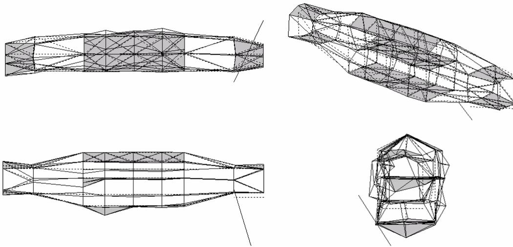
Figure 5 Operational Deflection Shape – 13.7Hz (factored frequency)
