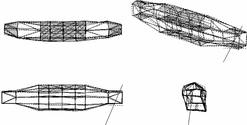
Figure 2 Lateral Bending Mode
