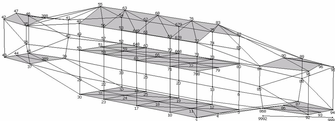
Figure 1 Measurement locations on the railcar
