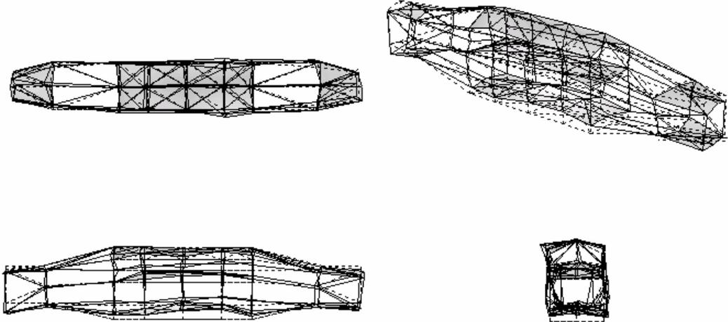
Figure 3 Vertical Bending Mode
