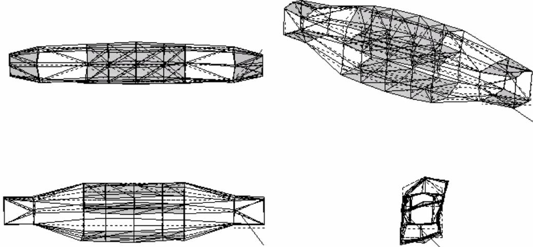
Figure 4 Whole Body Shear Mode
