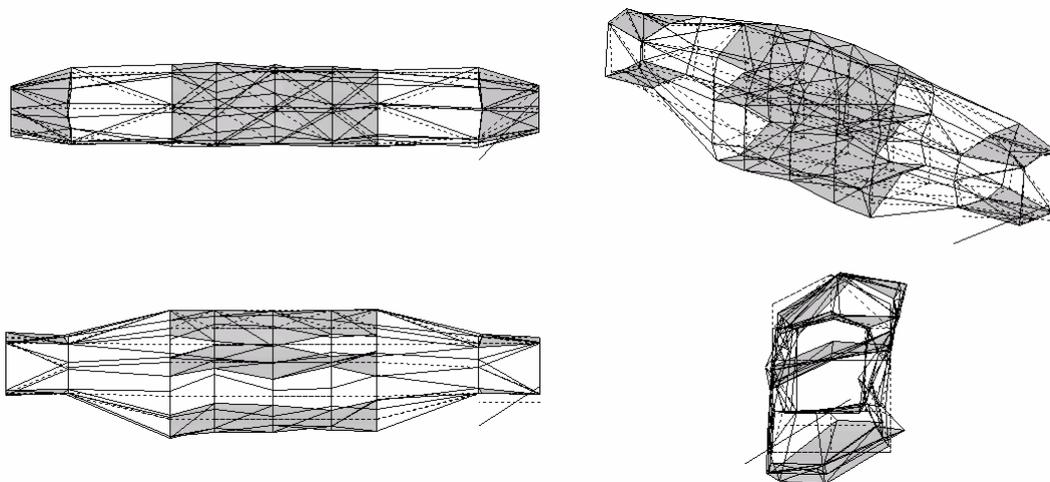
Figure 6 Operational Deflection Shape – 15.3Hz (factored frequency)
