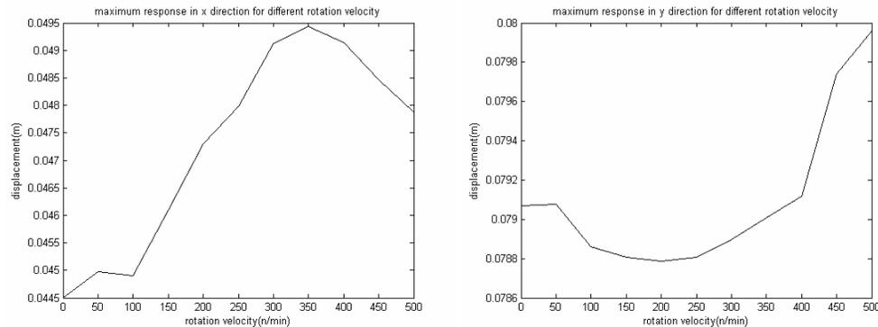
Fig.8 Shock response of the propulsion shaft for different rotation velocity
