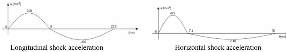
Fig.5 Shock acceleration
