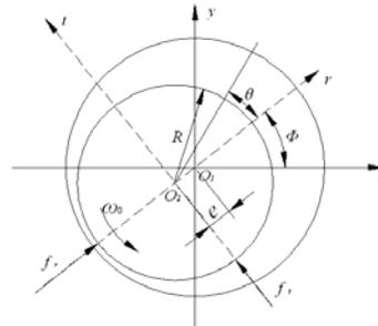
Fig.2 Coordinate of the oil film bearing
