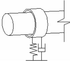
Fig.1 The oil film bearing
