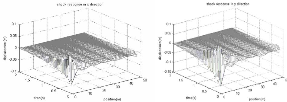
Fig.7 Shock response of the propulsion shaft
