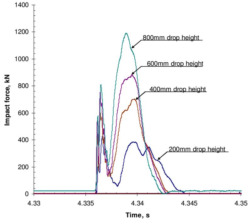
**Figure 7** Impact forces at different drop heights
