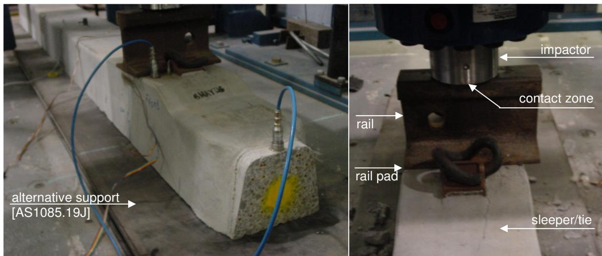
**Figure 4** Experimental setup
