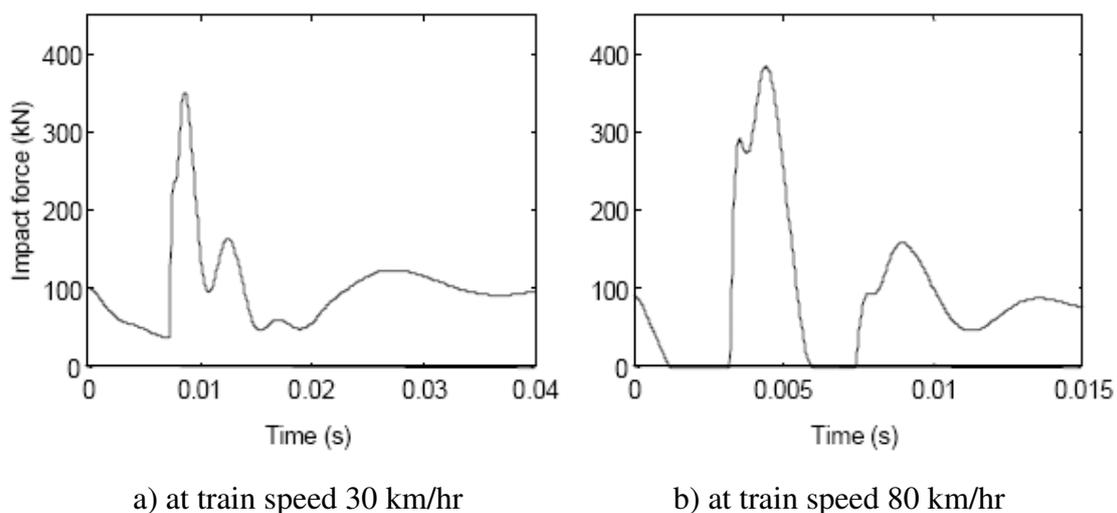
**Figure 3** Dynamic forces due to 2 mm rounded wheel flat [13]
