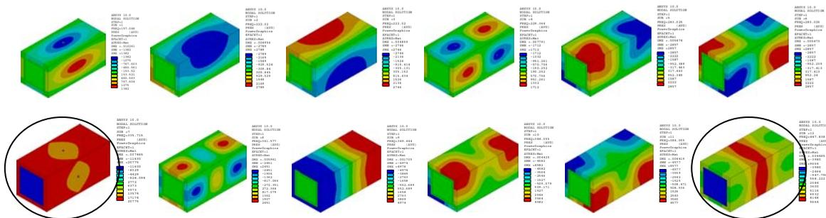
Fig.7. Eigenmodes of the fluid-structure system, synchronised modes are in the circle
