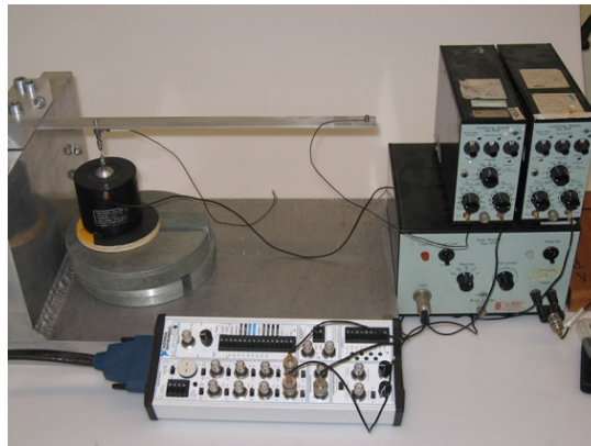
Figure 6. Measuring setup with clamped beam
