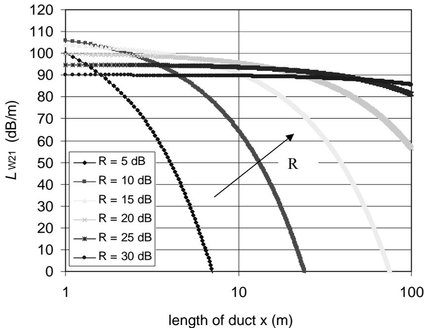
Figure 6 Distribution of sound power level  $L_{w21}$  along duct (related to sound power level at the beginning of the duct  $L_{w1} = 120$  dB,  $D = 400$  mm)
