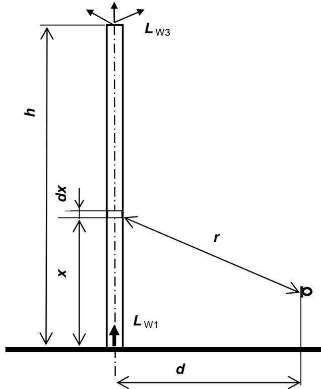
Figure 5 Distribution of sound from smoke stack
