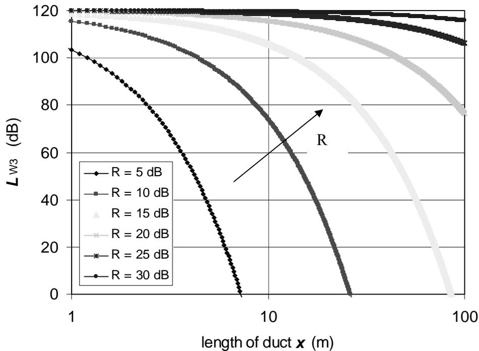
Figure 4 Diagram of sound emission from smoke stack ( $L_{W_1} = 120\text{dB}$ ,  $D = 400\text{ mm}$ )
