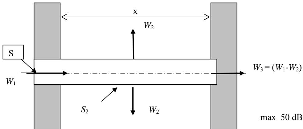
Figure 1 Diagram of noise emission from duct
