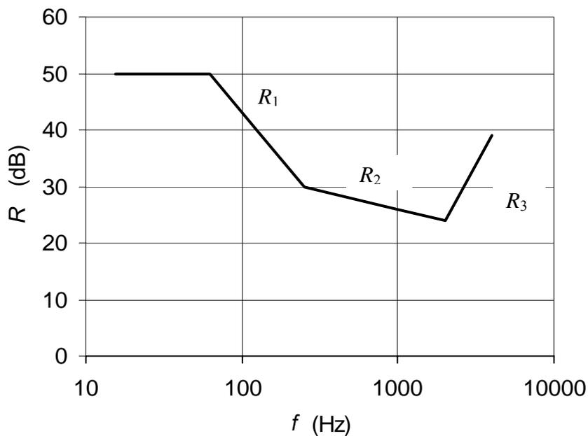
Figure 2 Spectrum of air transmission loss of a circular cross-section duct
