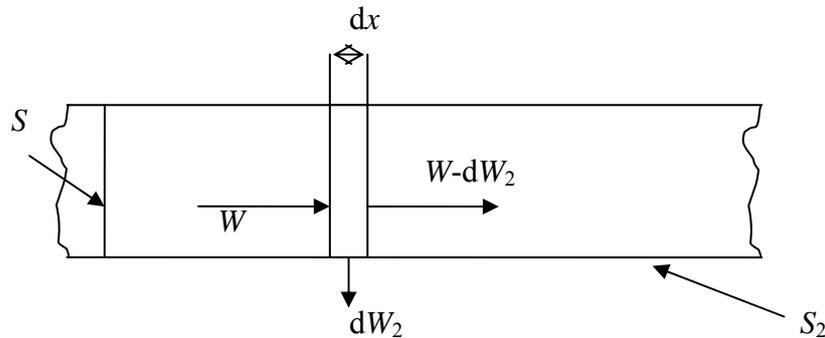
Figure 3 Diagram of sound propagation in a duct without transmission losses
