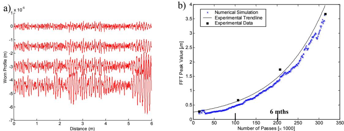
Figure 6. Measured and Simulated Profile Evolution. a) Initial measured profile and subsequent simulated profiles at 90,000 wheelset pass intervals, b) comparison of FFT corrugation peak growth.
