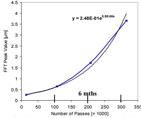
Figure 4. Growth of FFT Peak. (■) 109mm Peak Wavelength Value and (-) Trendline
