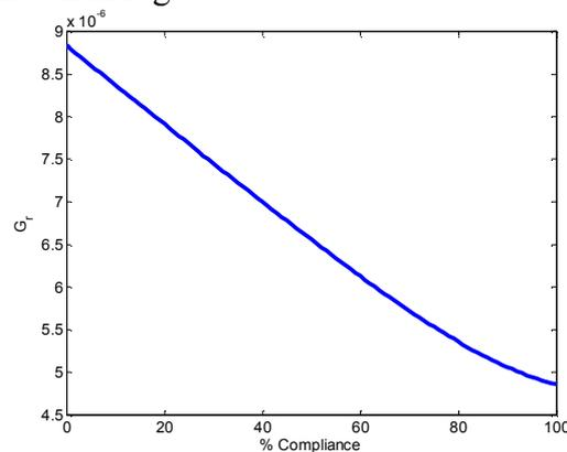
Figure 8. Corrugation Growth Rate for Different Levels of Driver Compliance.
