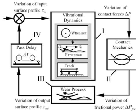
Figure 1. Feedback model for corrugation formation.
