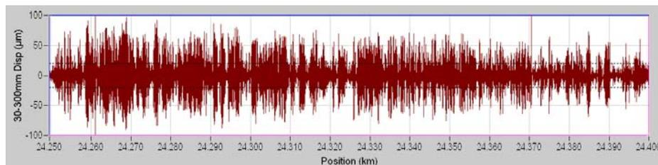
Figure 2. Measured profile of corrugated test section after Bandpass Filtering between 30 and 300mm.
