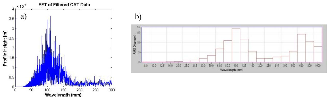
Figure 3. Wavelength spectrum of corrugated test section; a) FFT analysis, b) Third Octave analysis.
