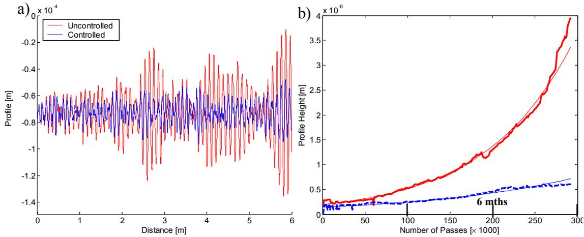
Figure 7. Comparison of corrugation growth under existing and controlled speed distributions; a) predicted profiles after 9 mths growth, b) FFT corrugation peak growth.
