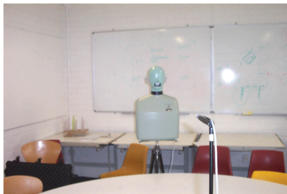
Figure 5. Modified HATS in the conference room
