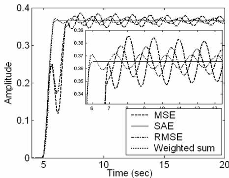
Figure 5: Response of vertical channel (leading edge only) with shaped commands for different objective functions ( $\sigma_s = 0.1$ )
