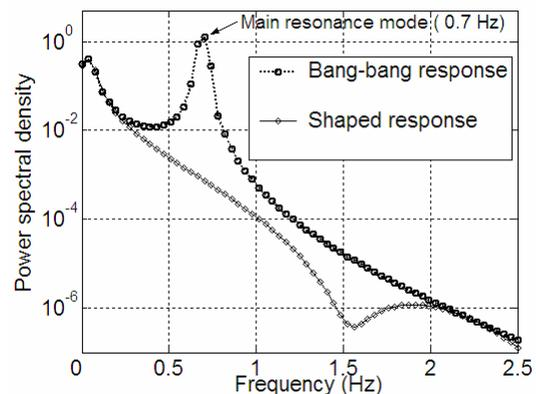
Figure 10: Response of vertical channel due to bang-bang signal and shaped command (frequency domain)
