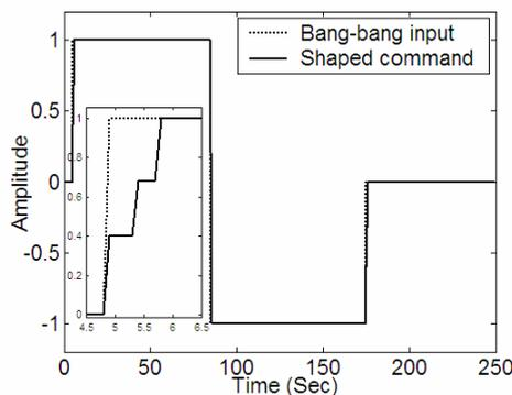
Figure 7: Bang-bang input and shaped command (time domain)
