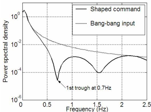
Figure 9: Bang-bang input and shaped command (frequency domain)
