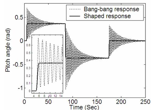
Figure 8: Response of vertical channel due to bang-bang signal and shaped command (time domain)
