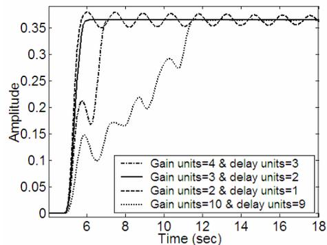
Figure 6: Leading edges of output response with command shapers having different numbers of gain and delay units.
