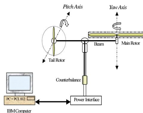
Figure 2: Schematic diagram of TRMS
