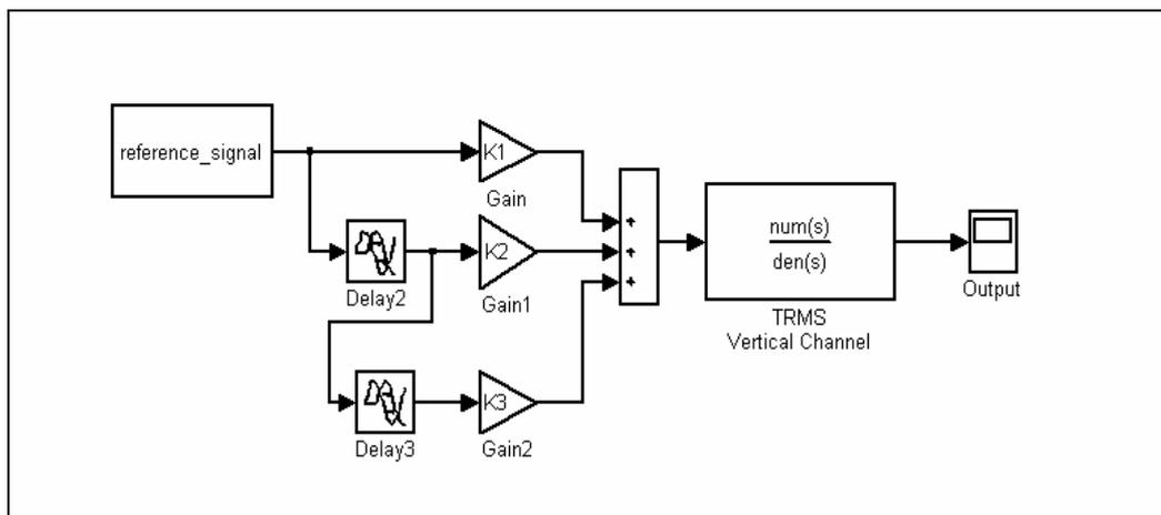
Figure 4: Simulink model of command shaping using gain and delay units
