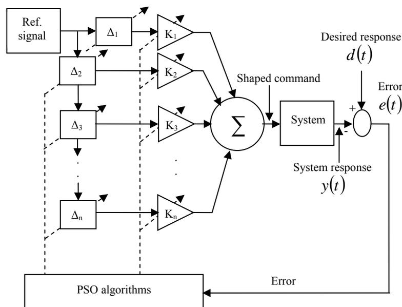
Figure 3: Proposed PSO-based command shaping scheme using gain and delay elements
