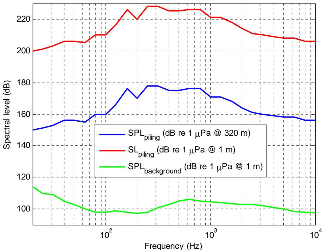
Figure 2. Sound pressure levels at 320 m (blue) and 1 m (red) of the piling activity as compared to the background noise in the area (green)
