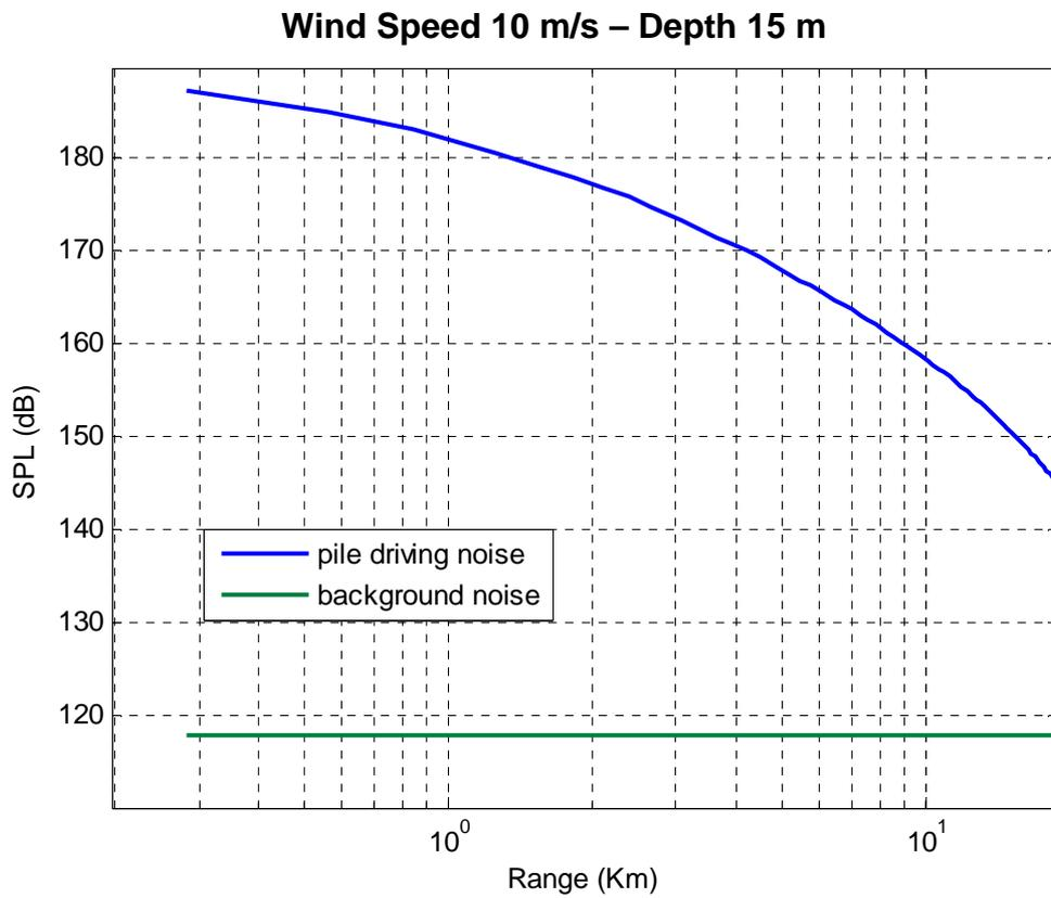
Figure 4. Spreading of piling noise (solid line) as compared to the background noise (dotted line) in the area
