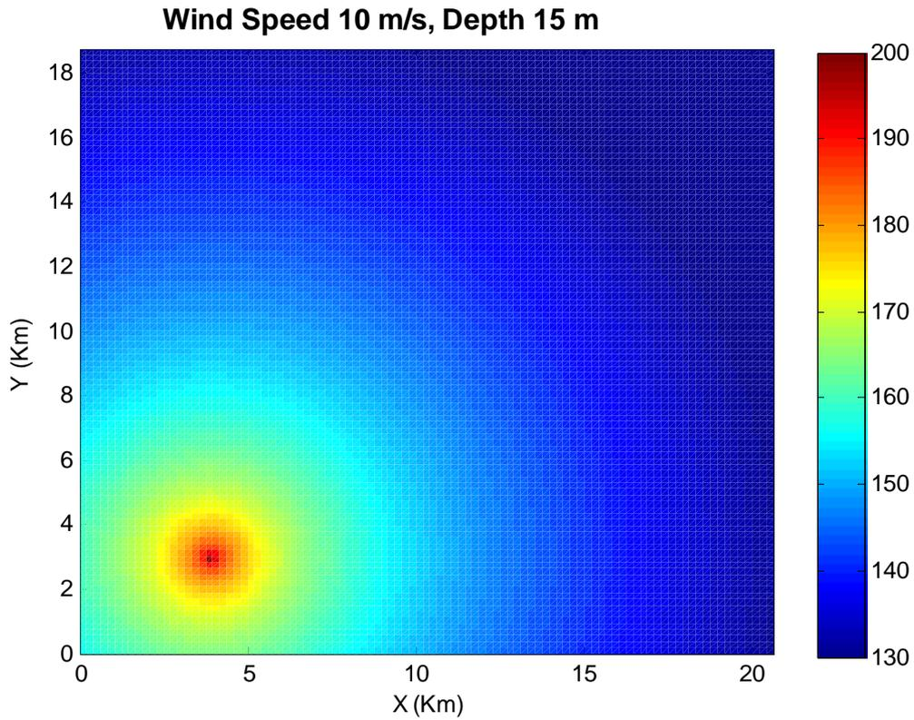
Figure 3. Overall noise map produced by piling activity in the area at half depth
