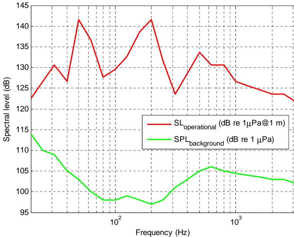
Figure 5. Spectral levels of operational noise (red) as compared to those of the background noise (green) in the area
