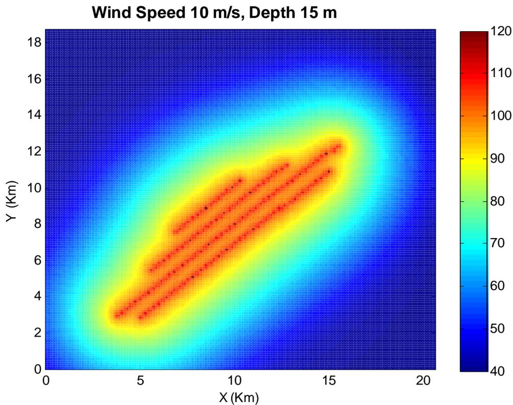
Figure 6. Map of the overall operational noise produced by 145 wind turbines in the area
