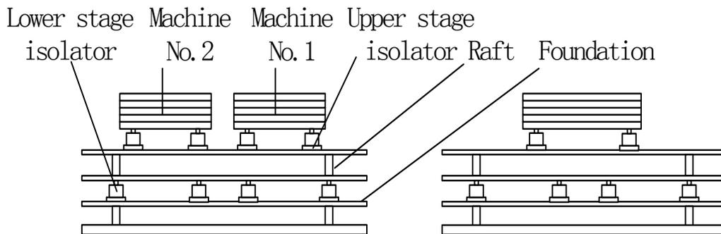
Figure 2. Model of the raft vibration isolation system
