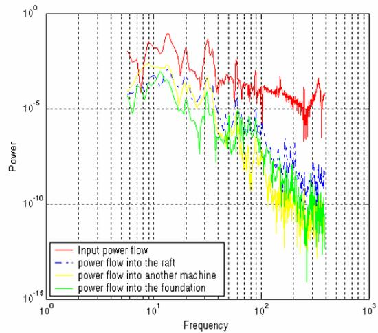
Figure 5 Power flow of the raft isolation system
