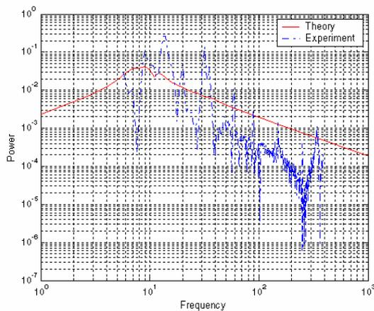
Figure 6. Power flow input to the vibration isolation system
