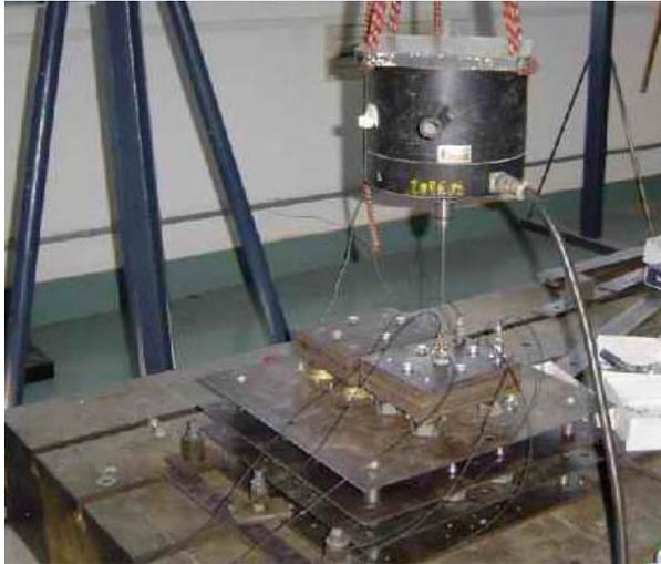
Figure 4. Power flow testing of the raft vibration isolation system
