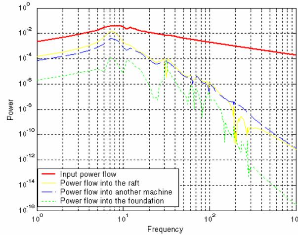
Figure3. Power flow of the elastically coupled vibration isolation system
