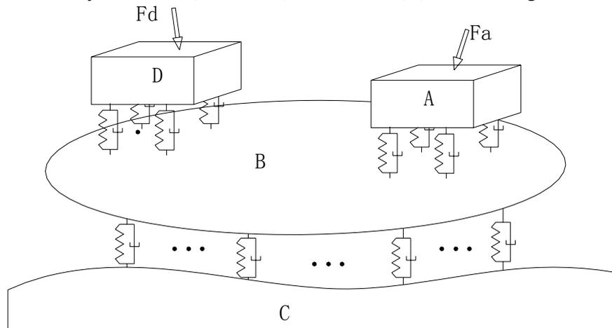
Figure 1. Three dimensional raft vibration isolation system
