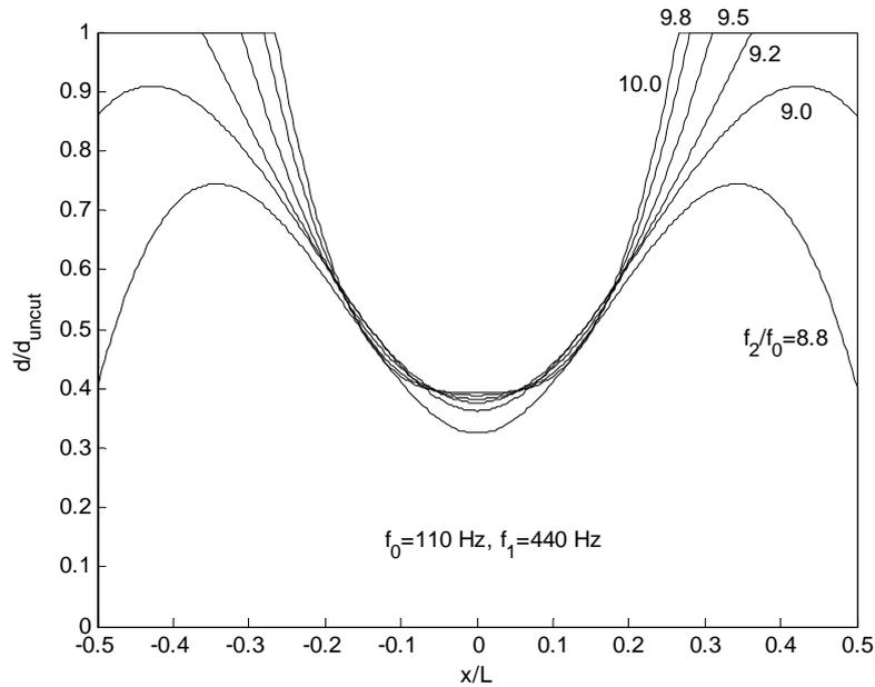
Figure 2. Predicted undercut geometries using cubic equation (13) and various  $\frac{f_2}{f_0}$  ratios.
