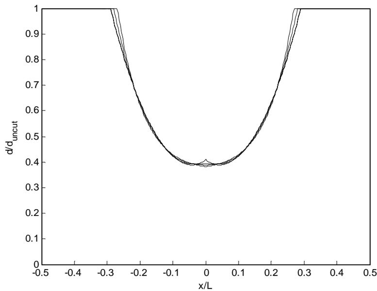
Figure 3. Predicted undercut geometries using equations (13-16),  $f_0 : \frac{f_1}{f_0} : \frac{f_2}{f_0} = 110:4:9.8$ .
