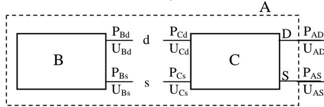
Figure 1. Joining beam sections B and C to give tip receptances of A
