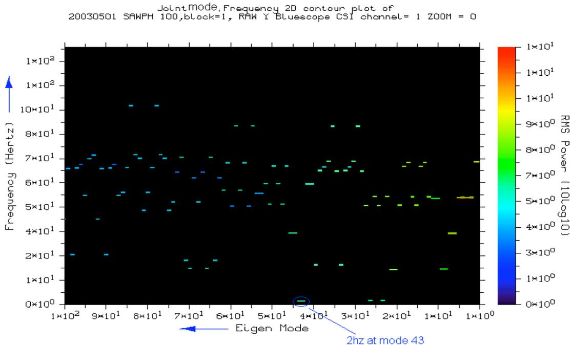
Figure4. Coal Reclaimer  $x$  Acceleration frequency, eigen-mode, RMS Power at 01/05/2003
