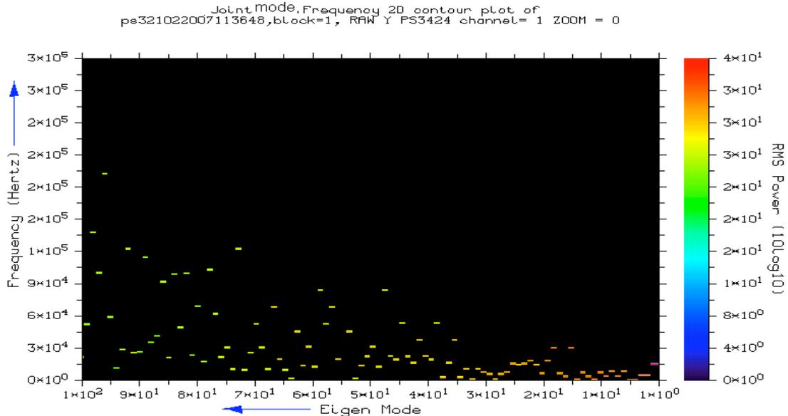
Figure7. Test-rig channel 1,  $x$  Acceleration frequency, eigen-mode, RMS Power at 21/02/2007
