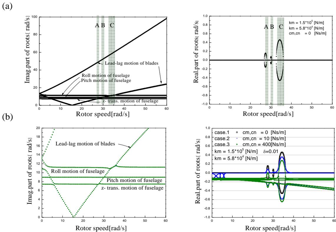
Figure 6 Stability diagram by linear modeling of spring & dashpot in landing gear
