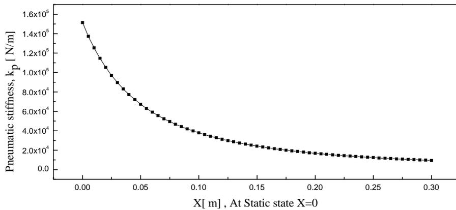
Figure 3. Pneumatic stiffness of gas in the upper chamber vs. absorber states
