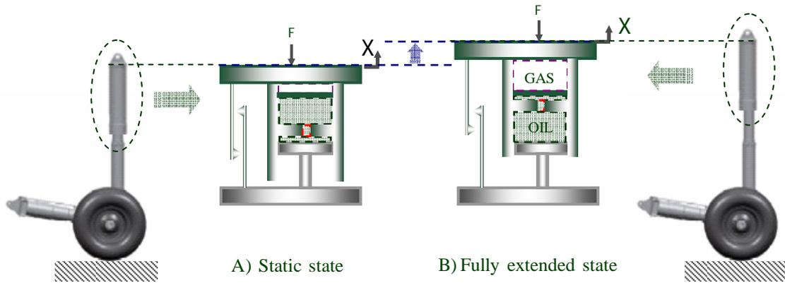
Figure 2. State variation of oleo-pneumatic shock absorber model
