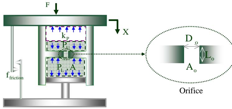
Figure 4. Schematic of oleo-pneumatic shock absorber model development.
