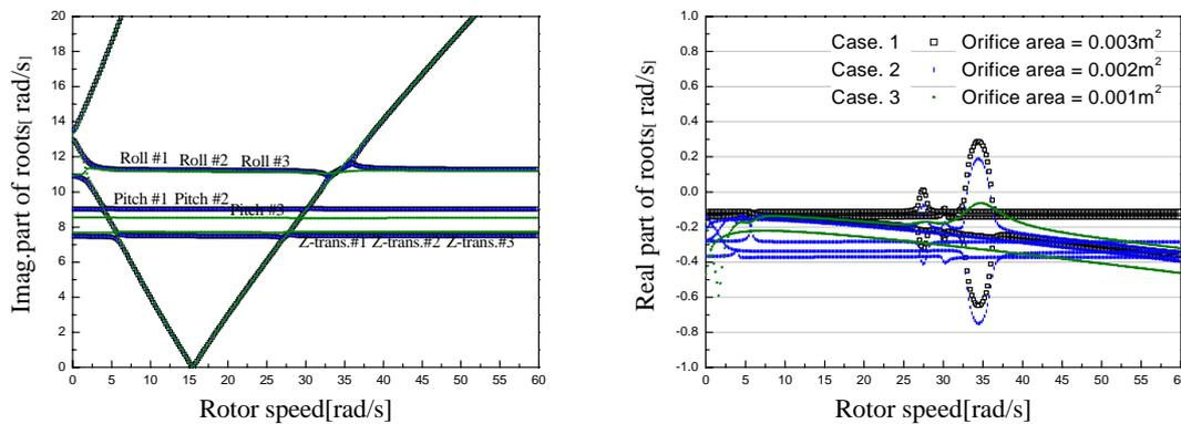
Figure 7 Stability diagram by nonlinear modeling of oleo-pneumatic shock absorber in landing gear (a) various static state (b) various orifice areas
