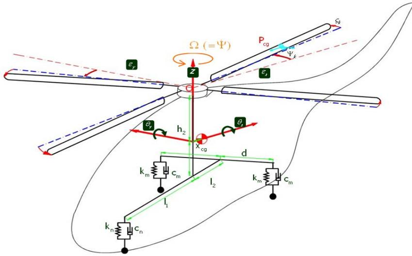
Figure 1. Schematic diagram of ground resonance model for helicopter
