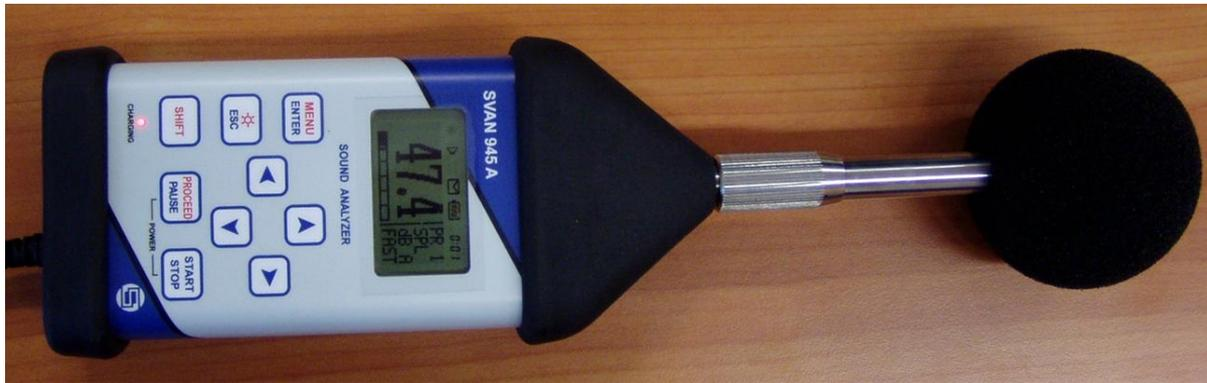
Figure 2. Overall view of meter SVAN 945A.
