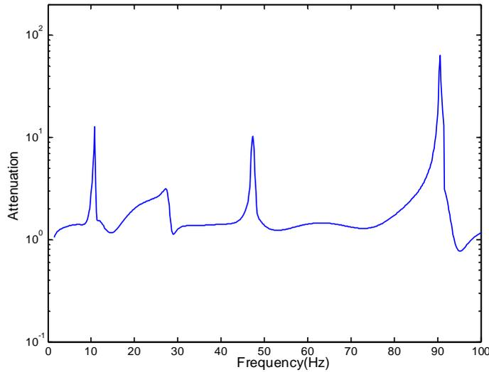
Fig. 7 Attenuation of bending wave propagating in a 4-cell periodic structure
