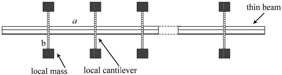
Fig.3 the periodic structure: beam attached with local cantilever-mass phonon structure
