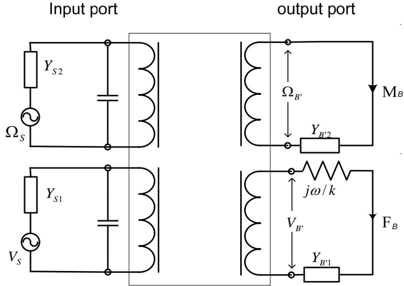
Fig.2 Equivalent circuit diagram to the model of a simple source mounted on load beam with isolators such as Fig. 1, based on an analogy model of 8-port network.
