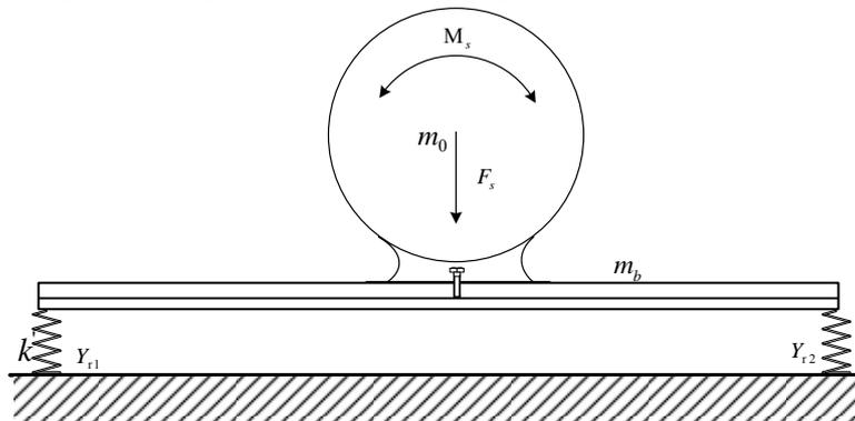
Fig.1 simple model of a source elastically mounted with supporting beam.
