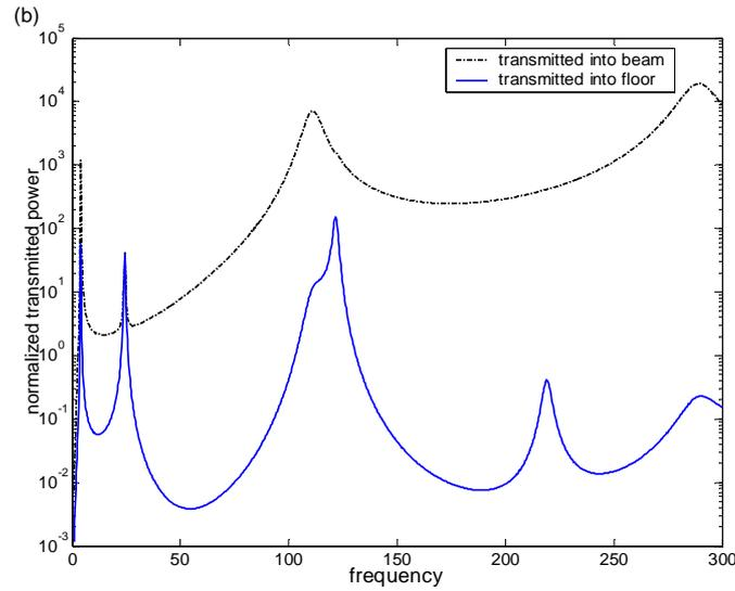
Fig. 5 The transmitted vibratory power from the elastically mounted simple source on load beam. (a) damping coefficient of isolator  $\dot{\eta}=0$ . (b) damping coefficient of isolator  $\dot{\eta}=0.005$ .
