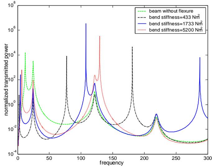
Fig. 4 The transmitted vibratory power from the elastically mounted simple source on the load beam of various bend stiffness.
