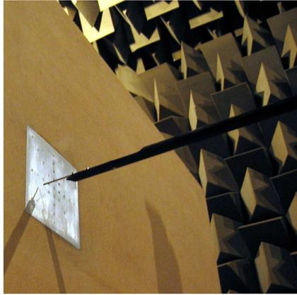
(a) microphone beam during measurement of a hologram position
