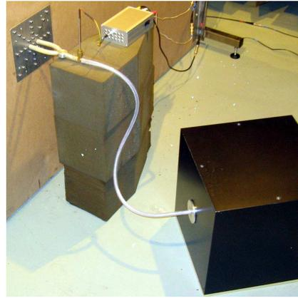
(b) isolated speaker connected to the backside of the baffle
