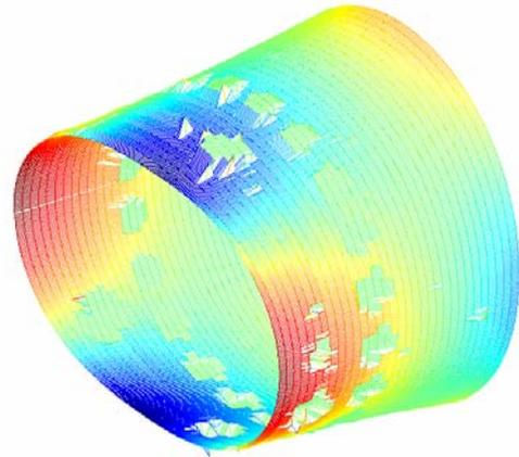
Figure 7 Scanning LDV measurement of cylindrical structure modeshape
