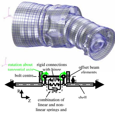
Figure 5 Typical joint in structural assembly
