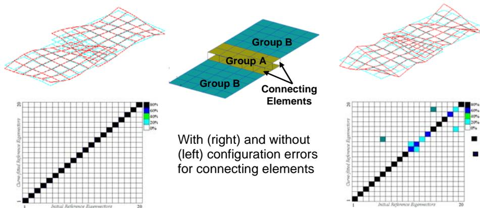
Figure 4 Example of model verification check
