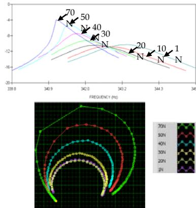
Figure 6 Evidence of non-linear behaviour
