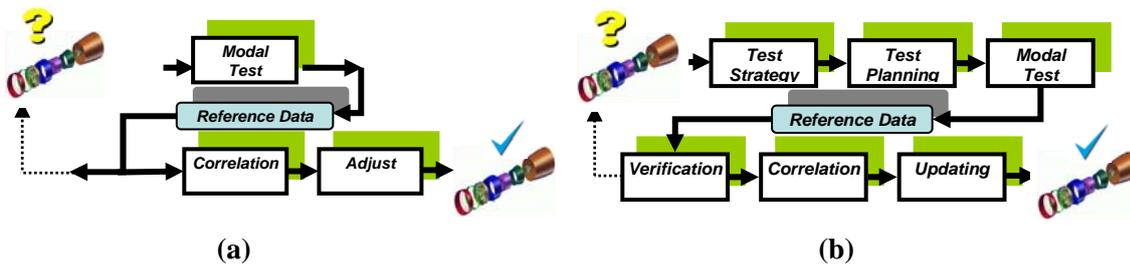
Figure 1 Schematics of model validation procedures (a) 1970s (b) 2000s
