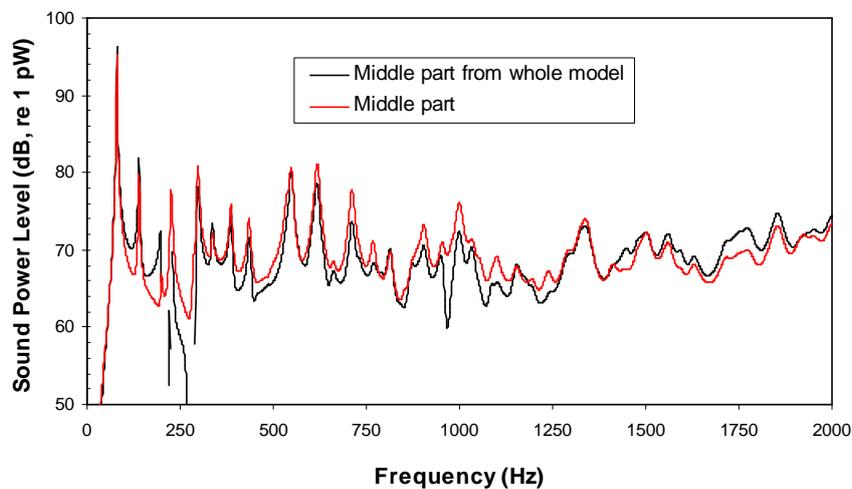
Figure 5. Sound power level spectra; separate middle part and middle part from the total model.
