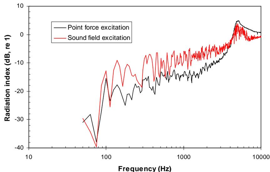
Figure 3. Radiation index spectra of different excitation mechanisms.
