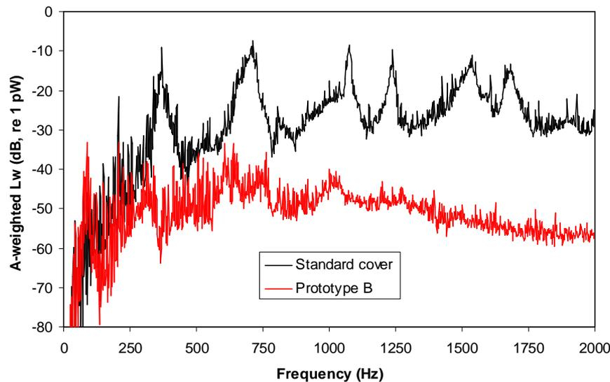
Figure 7. A-weighted sound power level spectra of standard cover compared to prototype B.
