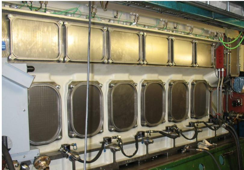
Figure 6. Measurement object equipped with prototype covers.
