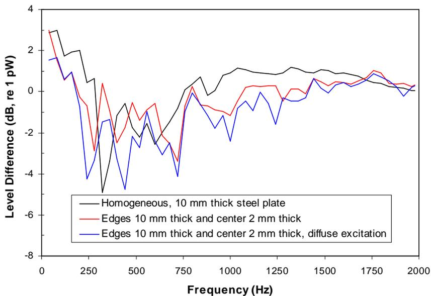
Figure 4. Deviation of the sound power levels calculated in parts from the result calculated as a whole.
