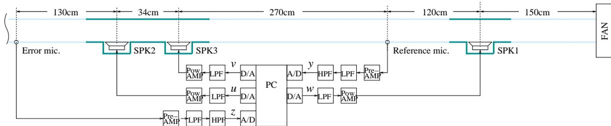
Figure 1. Experimental apparatus
