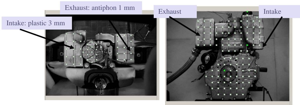
Figure 8. Vibrational mesh (left: top surface, right: front surface)
