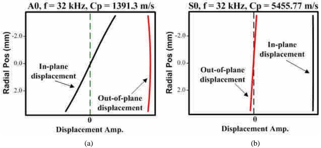
Figure 6. Mode shape of (a) A0 and (b) S0 mode in plate at 32 kHz [7].
