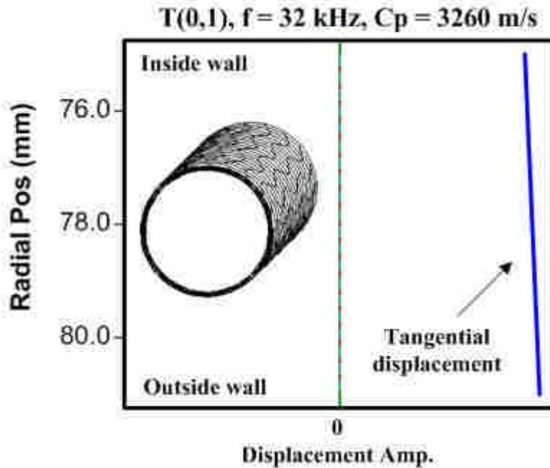
Figure 5. Mode shape of T(0,1) mode in pipe at 32 kHz [7].
