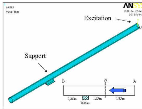
Figure 1. FEM model of a pipe with a longitudinal welded support.
