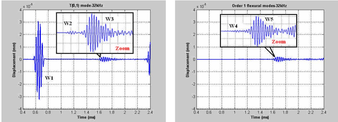
Figure 3. The time history of (a) T(0,1), (b) F(1,2) and F(1,3) mode at monitor line C.
