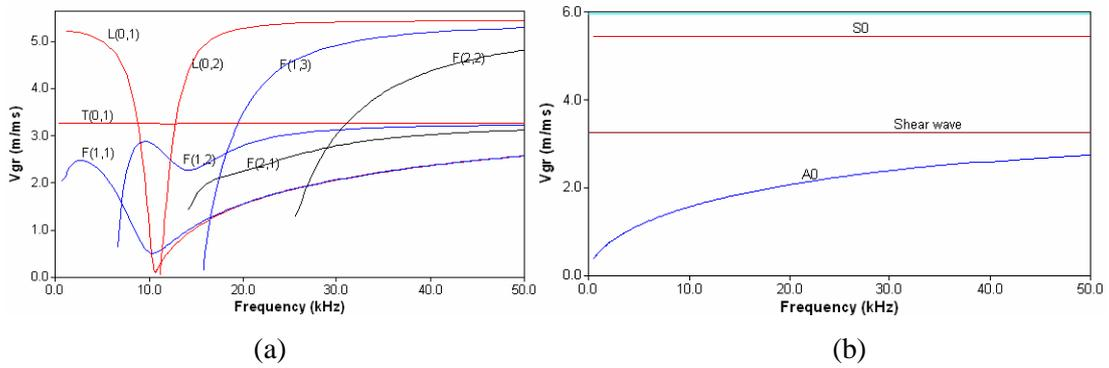
Figure 4. Group velocity dispersion curve of (a) a 6 inch pipe and (b) a 7 mm thick steel plate [7].
