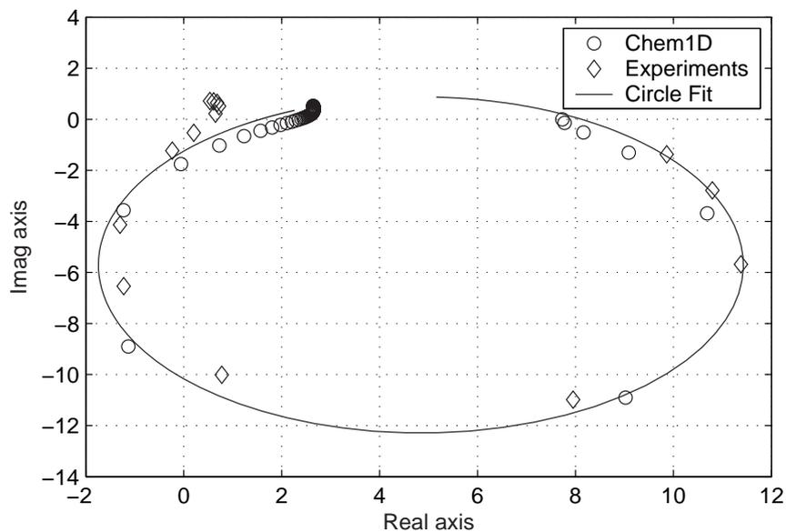
Figure 2. Nyquist plot for the flame transfer function ( $\phi = 0.8$  and  $\bar{u}_u = 14(\text{cm/s})$ )
