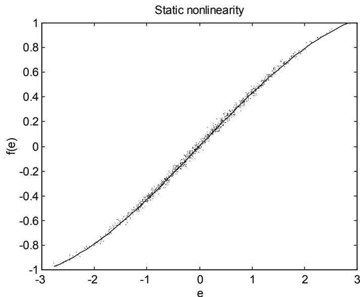
Figure 4. Static nonlinearity (plant - solid line; identified model - dotted line).
