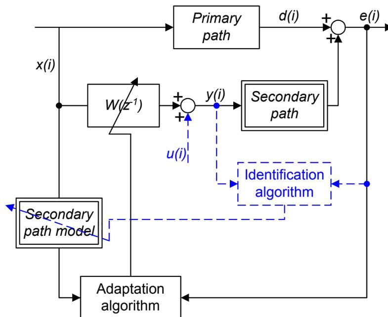
Figure 1. Adaptive feedforward ANC system.
