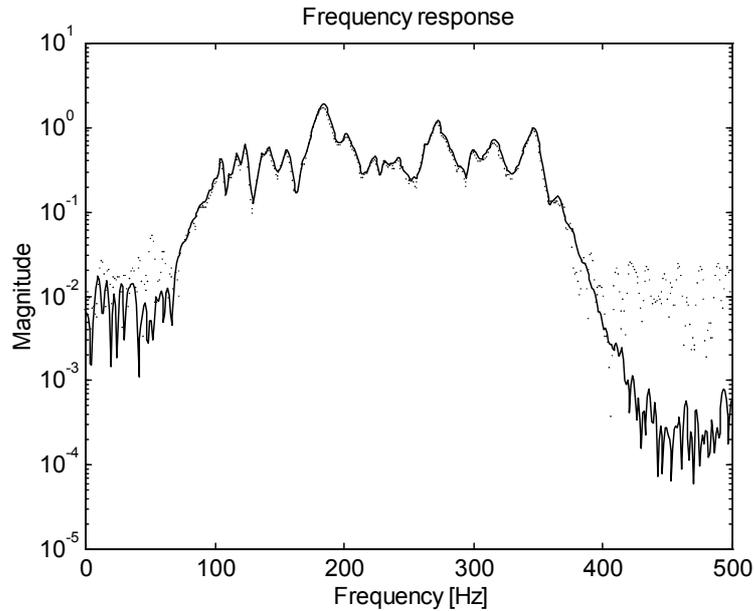
Figure 3. Frequency response magnitude of linear dynamic part of the Wiener system (plant - solid line; identified model - dotted line).
