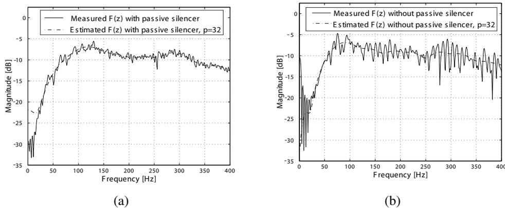
Figure 7. Frequency response functions of the measured (solid line) forward path  $F(z)$  with 256 coefficients and the estimated (dash-dotted line) forward path  $\hat{F}(z)$  with 32 coefficients in (a) with passive silencer and in (b) without passive silencer.
