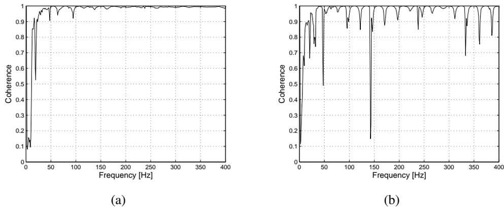
Figure 5. Coherence between the reference signal  $x(n)$ , and the primary noise signal  $d(n)$ , in (a) when using the passive silencer and in (b) when *not* using the passive silencer.
