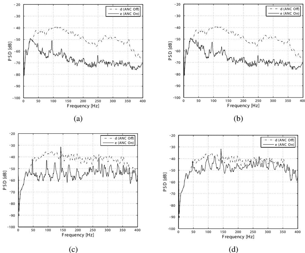
Figure 4. Power spectral density of the primary noise signal  $d(n)$  (dash-dotted), and the error signal  $e(n)$  (solid), when using (a) the passive silencer and a feedback neutralization filter, (b) the passive silencer and no feedback neutralization filter, (c) no passive silencer and a feedback neutralization filter, and (d) no passive silencer and no feedback neutralization filter.
