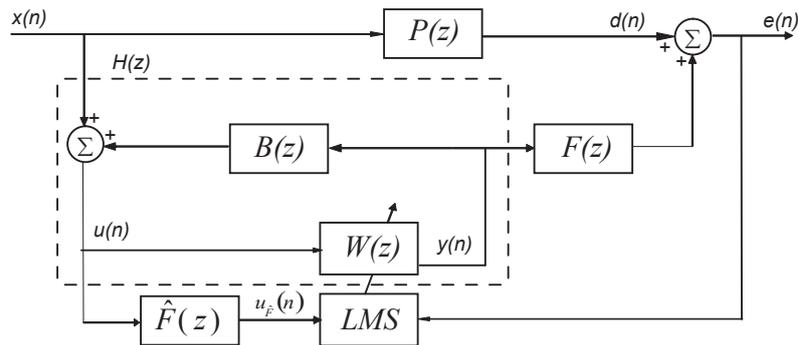
Figure 2. Block diagram of an ANC system with acoustic feedback using the filtered-x algorithm. The signal  $x(n)$  is the reference signal related to the primary noise source and the signal  $u(n)$  is the reference microphone signal including the contribution based on the acoustic feedback.
