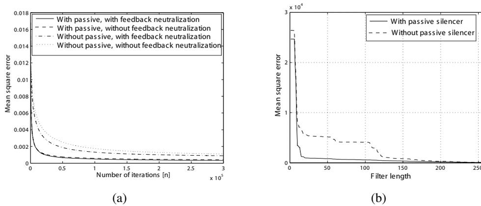
Figure 6. In (a) mean square error as a function of number of iterations with the ANC system in operation. In (b) mean square error as a function of filter length when estimating the forward path using the LMS algorithm.
