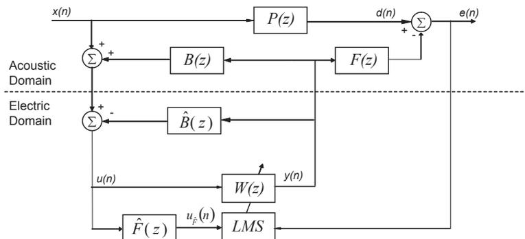
Figure 3. Block diagram illustrating the construction of the ANC system used in the simulations.
