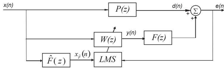
Figure 1. Block diagram of a feedforward ANC system without acoustic feedback using the filtered-x LMS algorithm.
