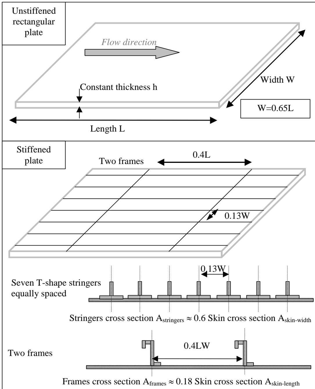
Figure 1. Unstiffened and stiffened plate characteristics – Frames, stringers and skin are all made of the same isotropic material.
