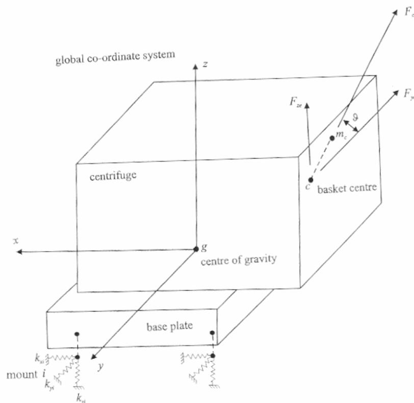
Figure 1. Centrifuge assembly model.
