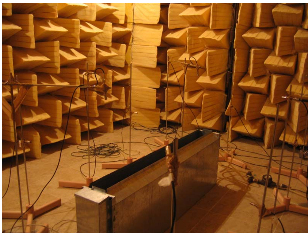
Figure 3. An example of a sound power measurement using ISO 2744 inside a semi anechoic room.
