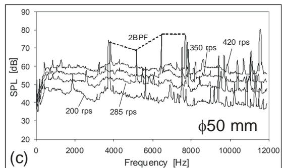
Figure 6. Noise spectra of suction unit with a vaned diffuser at three rotational speeds ( $n = 205, 285$  and  $420$  rps) and ten different flow regimes (orifice diameter  $\phi 0, \phi 6.5, \phi 10, \dots$  to  $\phi 50$  mm); BPF – blade passage frequency
