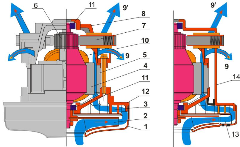
Figure 1. Single stage dry suction unit: *a)* without vaned diffuser and *b)* with vaned diffuser; 1-blower cowl, 2-rotor of the blower, 3-return passages, 4-stator of the EM, 5-rotor of the EM, 6-collector, 7-commutator brushes, 8-yoke B, 9- and 9'-air jets, 10-windings, 11-ball bearings, 12-yoke A, 13-diffuser vanes, and 14-cylindrical metal shield
