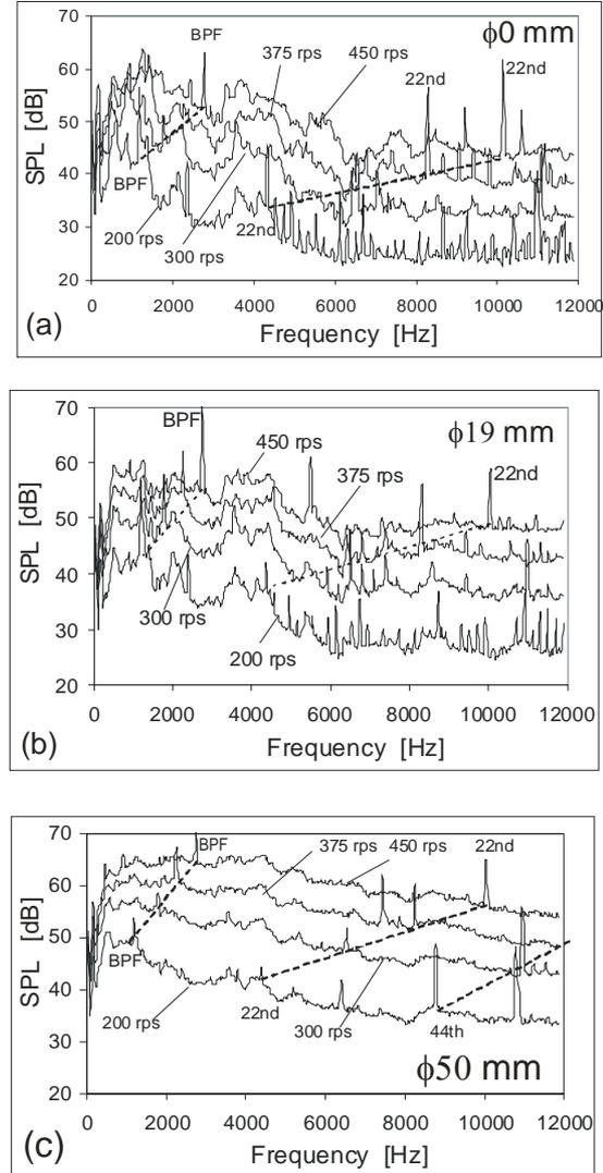
Figure 5. Noise spectra of suction unit without vaned diffuser at four rotational speeds ( $n = 200, 300, 375$  and  $450$  rps) and three different flow regimes: *a*) at zero flow rate (orifice  $\phi 0$  mm), *b*) at BEP (orifice  $\phi 19$  mm) and *c*) at free delivery (orifice  $\phi 50$  mm)
