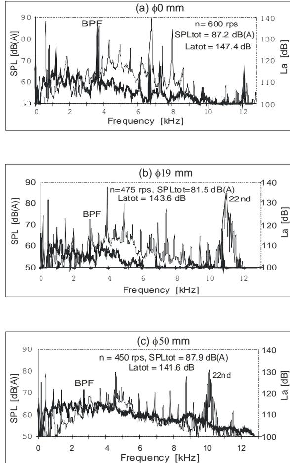
Figure 3. Comparison between noise spectra (thick curve) and vibration spectra (thin curve) of suction unit without vaned diffuser at constant voltage supply (230 V) and different flow regimes: *a*) at zero flow rate (orifice  $\phi 0$  mm), *b*) at BEP (orifice  $\phi 19$  mm) and *c*) at free delivery (orifice  $\phi 50$  mm);  $n$ -rotational speed, BPF-blade passage frequency,  $SPL_{tot}$ -total sound pressure level,  $L_{atot}$ -total level of vibration velocity
