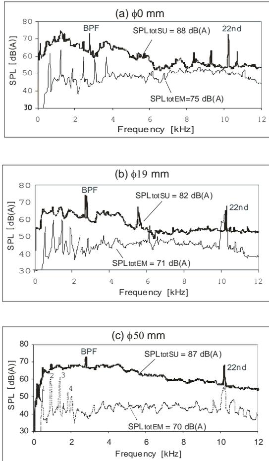
Figure 2. Noise spectra of complete suction unit without vaned diffuser (thick curve) and with dismantled rotor of the blower (thin curve) at constant voltage supply (230 V) and different flow regimes: *a*) at zero flow rate (orifice  $\phi 0$  mm), *b*) at BEP (orifice  $\phi 19$  mm) and *c*) at free delivery (orifice  $\phi 50$  mm);  $SPL_{totSU}$ -total sound pressure level of the suction unit,  $SPL_{totEM}$ -total sound pressure level of the EM
