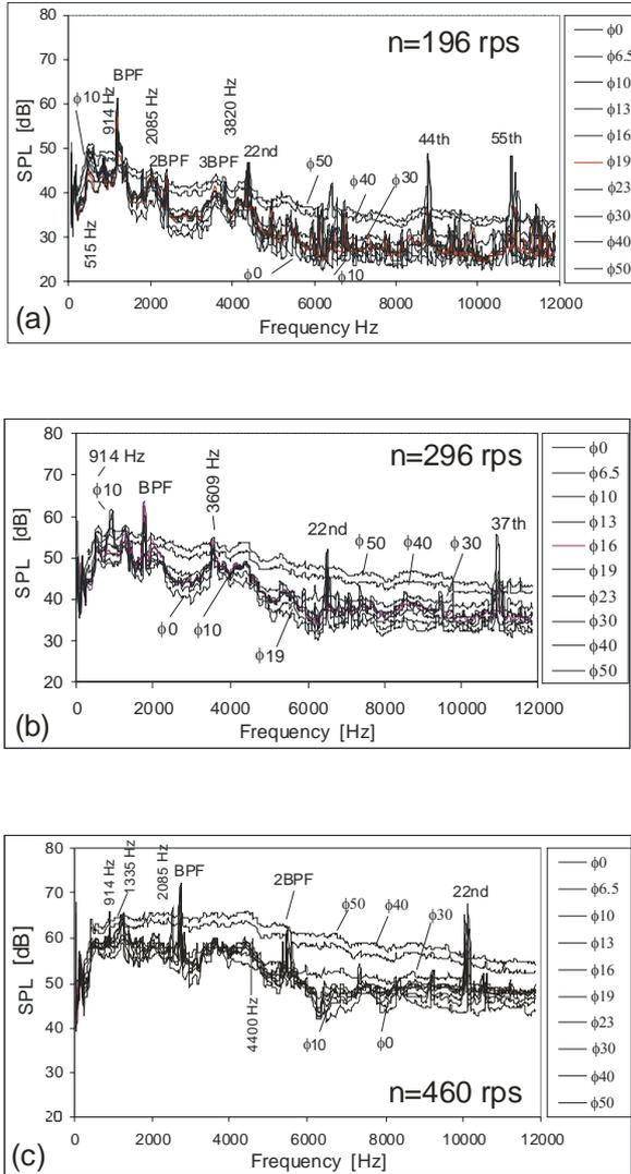
Figure 4. Noise spectra of suction unit without vaned diffuser at three rotational speeds ( $n = 196, 296$  and  $420$  rps) and ten different flow regimes (orifice diameter  $\phi 0, \phi 6.5, \phi 10, \dots$  to  $\phi 50$  mm)
