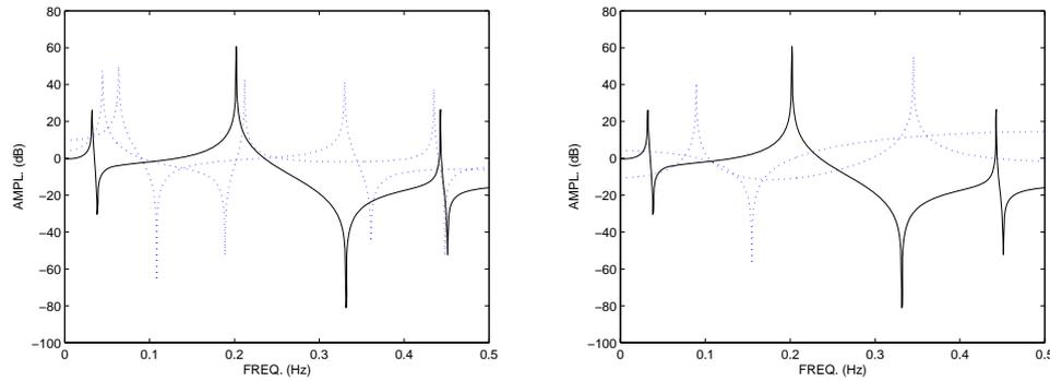
Figure 1. (a) Left - Scalar transmissibilities (dotted lines) for different loading conditions cross at the resonances frequencies. (b) Right - Multivariable transmissibilities (dotted lines) for different loading conditions do not cross at the resonances frequencies. The solid line is a frequency response function.
