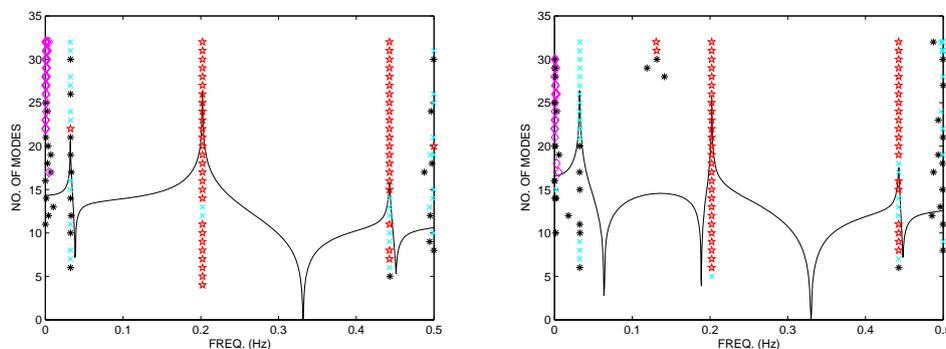
Figure 3. (a) Left - Stabilization chart obtain from a frequency response function. (b) Right - Stabilization chart obtain from a “virtual” frequency response function.
