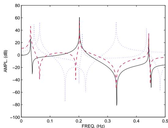
Figure 2. Solid line: a frequency response function. Dotted lines: two “virtual” scalar transmissibilities. Dashed line: a “virtual” frequency response function.
